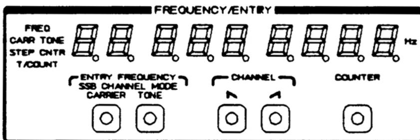
4.3 Frequency/Entry Group -On the upper RH side of the front panel is the frequency/entry sub-panel. This panel will usually display the frequency that the instrument is tuned to. It will display during frequency entry frequencies being entered by the instrument’s keyboard in KHz or Hz. This frequency will be the center RF frequency of the selected band pass filter except when in the SSB channel measurement modes.
