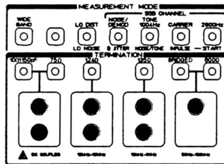
The termination sub panel is also located on the lower LH of the control panel. This panel is used to select the input termination for an input signal. The 50 or 75 ohm unbalanced input on the LH side of the panel is the only ones useful for radio work and used in the examples of this document. The others use nonstandard RF circuit impedances and are for telephone applications. See Chapter 3 for a complete description on how to connect to the unbalanced low impedance input.
