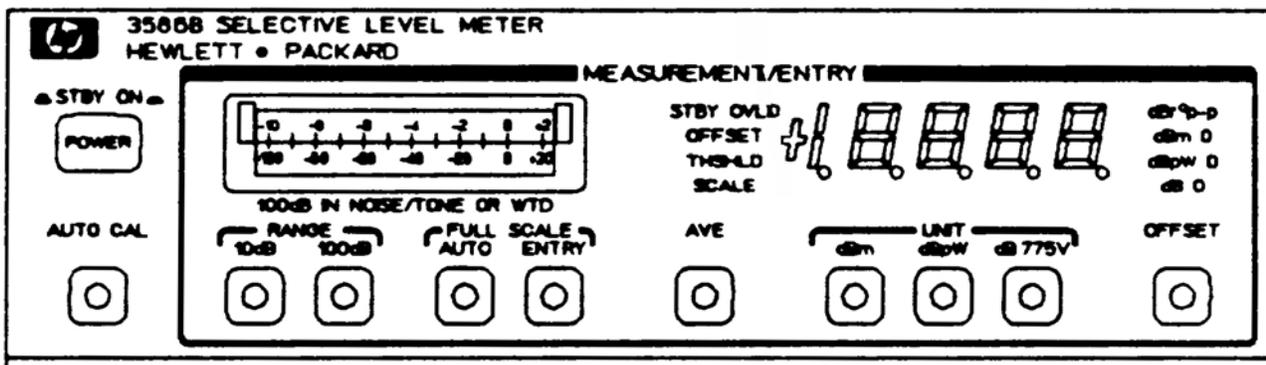
4.2 Measurement/Entry Group - On the upper LH is the measurement/entry sub panel, which is used for displaying the power or voltage measurements and their units on a LED display. The measuring range and range full scale range value is set using its buttons. Set the range by pressing [10db] and the full scale range limit by pressing [AUTO] for the automatic mode.
