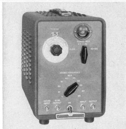
Fig. 3. Panel view of new hp-Model 512A. Dual type indicator tube is used to indicate both preselector tuning and output voltage level.
