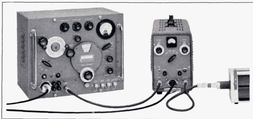
Fig. 1. New -hp- Model 491A 2-4 kmc Traveling-Wave Tube Amplifier (center) used with -hp- 616A UHF Signal Generator to form 1 watt signal source. Ten milliwatt TWT amplifier is similar in appearance to 1 watt unit shown.
