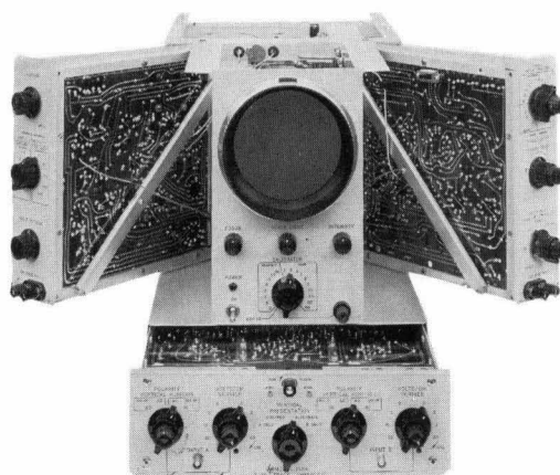
Fig. 13. Model 150A has been designed to afford high degree of accessibility to parts as indicated by above view of instrument with cabinet removed.
