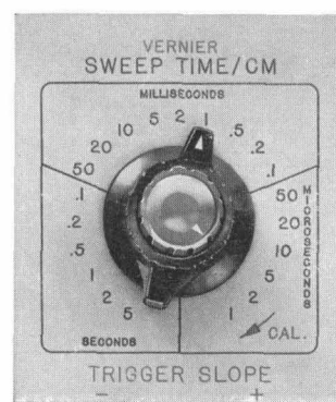
Fig. 4. To simplify sweep selection, sweep time selector is a single, direct-reading control. Concentric vernier enables continuous variation between steps.
