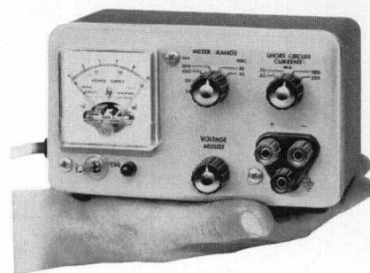
Fig. 1. —hp— Model 721A power supply provides 0 to 30 vdc at currents up to 150 ma. Maximum current available can be set by panel switch to minimize accidental overloading of sensitive external circuits.
