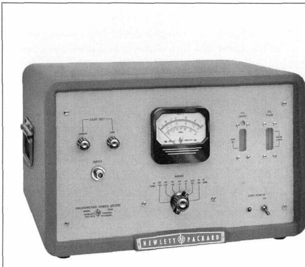
Fig. 1. New -hp- Model 434A Calorimetric Power Meter measures powers between a few milliwatts and 10 watts at frequencies from dc to 12.4 kilomegacycles. Self-balancing type circuitry makes operation automatic and gives reading in less than 5 seconds. Instrument is provided with 50-ohm coaxial input.
