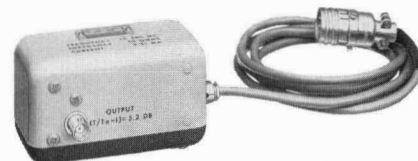
Fig. 2 (above). New Model 343A diode type VHF Noise Source provides flat noise output up to 600 megacycles without tuning for convenient testing of 50-ohm input receivers. Internal matching network compensates for transit-time effects in diode.
