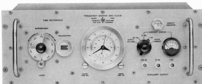
Fig. 1. New -hp- Model 113AR Frequency Divider and Clock simplifies intercomparison of local frequency standards with national standards via broadcast time signals and increases resolution with which such comparisons can be made. Use of instrument with suitable local frequency standard also permits time to be kept on a local basis to within a millisecond. Instrument is fully transistorized and designed with fail-safe provisions.
