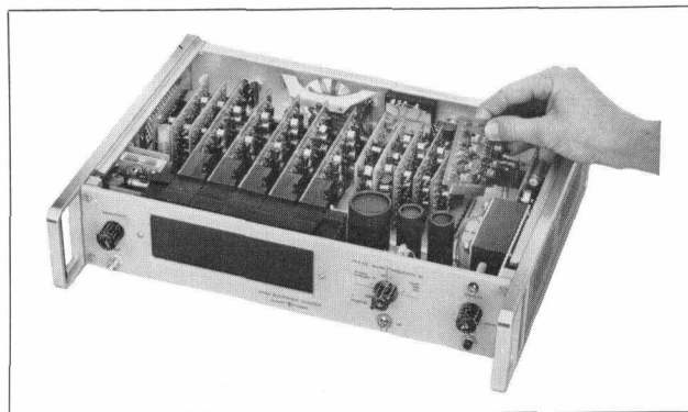
Fig. 10. Circuitry in new counters is built in plug-in modules.
