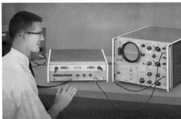
Fig. 1. New -hp- Model 8614A Signal Generator operates from 800 to 2400 Mc and provides outputs up to 10 to 60 mw. Generator is designed to provide leveled output, is also capable of being sine-wave modulated.
