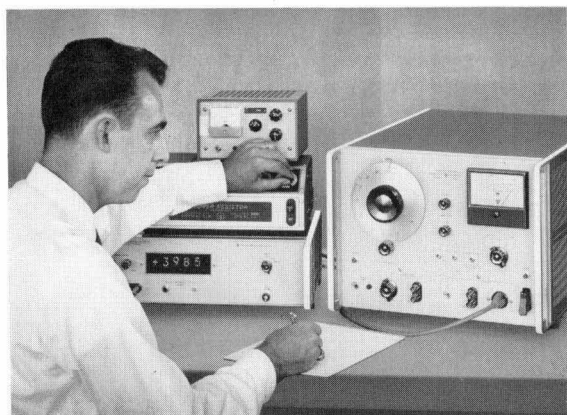
Fig. 1. Hewlett-Packard Model 4301A Variable Frequency Power Supply furnishes up to 250 volt-amperes at frequencies from 40 to 2000 cps. Output voltage is continuously adjustable from 0 to maximum of 130 or 260 volts. Unit also can serve as excellent line isolator.
