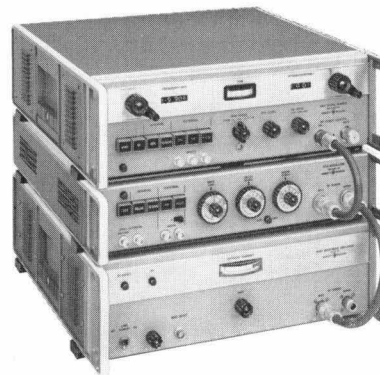
Fig. 13. Combination of new Model 8614A Signal Generator, 8714A Modulator, and 489A TWT Amplifier comprise high-performance signal generator with output of 1 watt.
