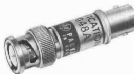
Fig. 7. Accessory feed-through termination has built-in 50-ohm resistance for terminating amplifier output while providing an output connection for external high impedance circuits.
