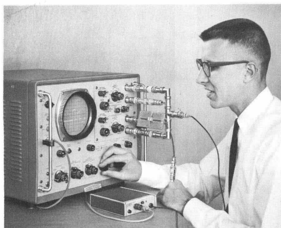
Fig. 1. New Model 188A dual-channel plug-in for -hp- Sampling Oscilloscope permits viewing signals of 90 picoseconds rise time, i.e., to above 4 gigacycles in frequency (to 8 Gc at reduced sensitivity). Plug-in is designed to view signals on 50-ohm lines by bridging line so that measured circuit is not disrupted.
