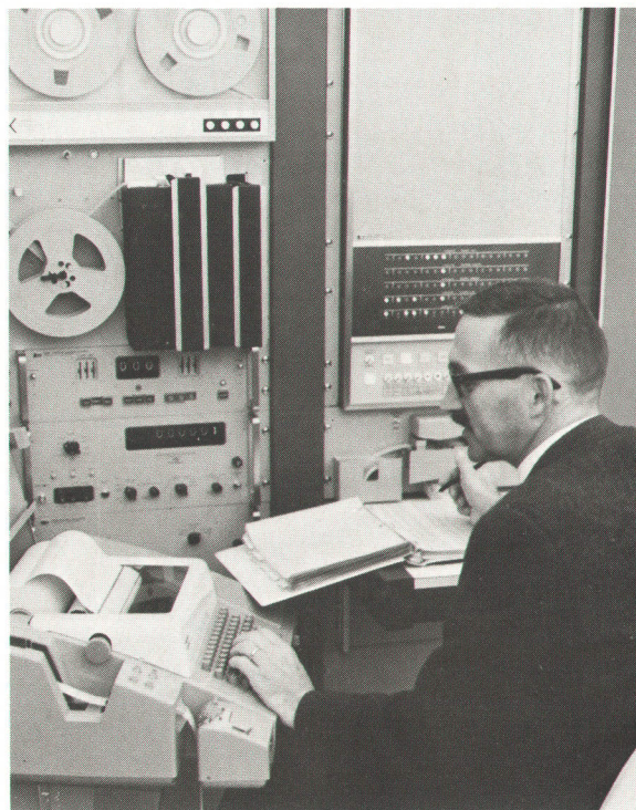
Fig. 1. Computing data acquisition system can be used in a variety of scientific and industrial applications, including jet engine testing (see Fig. 2).
