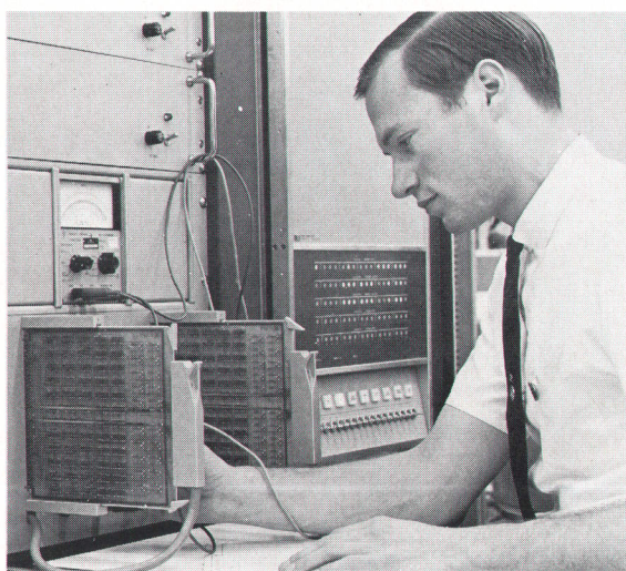
Fig. 5. —hp— 2116A Computer pretests logic cards for other —hp— 2116A Computers. Tests take only minutes per card, would take months without computer. Computer also keeps statistics for quality control.
