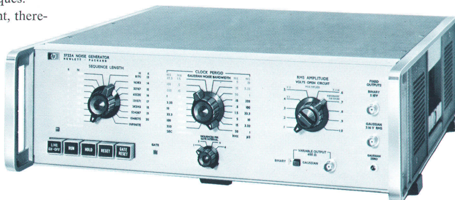
Fig. 1. A precision digital instrument, Model 3722A Noise Generator synthesizes repeated pseudo-random noise-like patterns or non-repeating random noise. Binary (two-level) and Gaussian (multi-level) outputs are generated. Amplitudes and bandwidths of outputs and lengths of pseudo-random patterns are variable.
