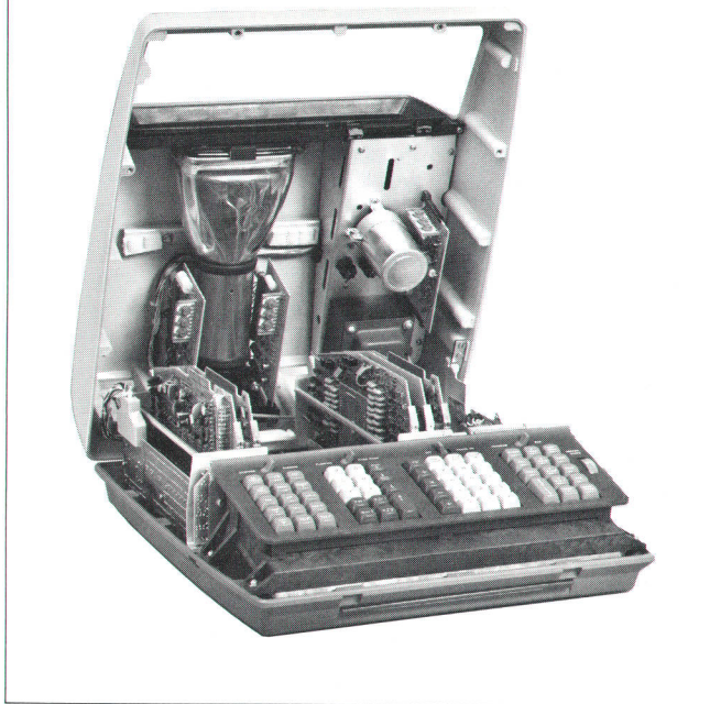
Fig. 5. Internal adjustments of the calculator are easily accessible by removing a few screws and lifting the top.
