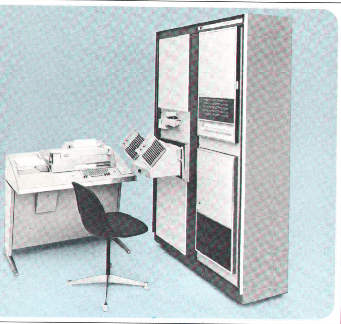
Fig. 1. Model 2060A Digital Logic Module Test System can give most production logic modules a thorough functional test in less than 30 seconds. It is programmed in AuTest, a special simplified language. Once programmed, it can be used by unskilled operators.
