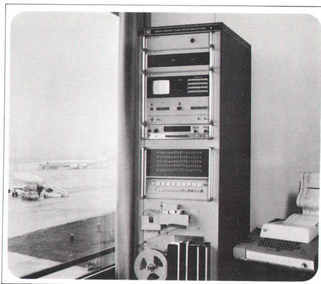
Fig. 4. The central processor can scan each noise monitoring terminal once each second, process the data, and present the results in the optimal form for evaluation by relatively untrained personnel. It can be adapted to future regulations and noise evaluation methods simply by changing programs.
