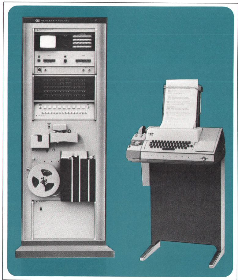
Fig. 1. Model 80501A Audio Data Processor consists of a real-time audio spectrum analyzer (with CRT) which measures the frequency spectra of audio-frequency inputs, a digital computer which processes the measured spectra, and peripheral devices. A typical application is aircraft noise analysis and evaluation. Real-time processing gives results almost immediately so appropriate action can be taken if required.
