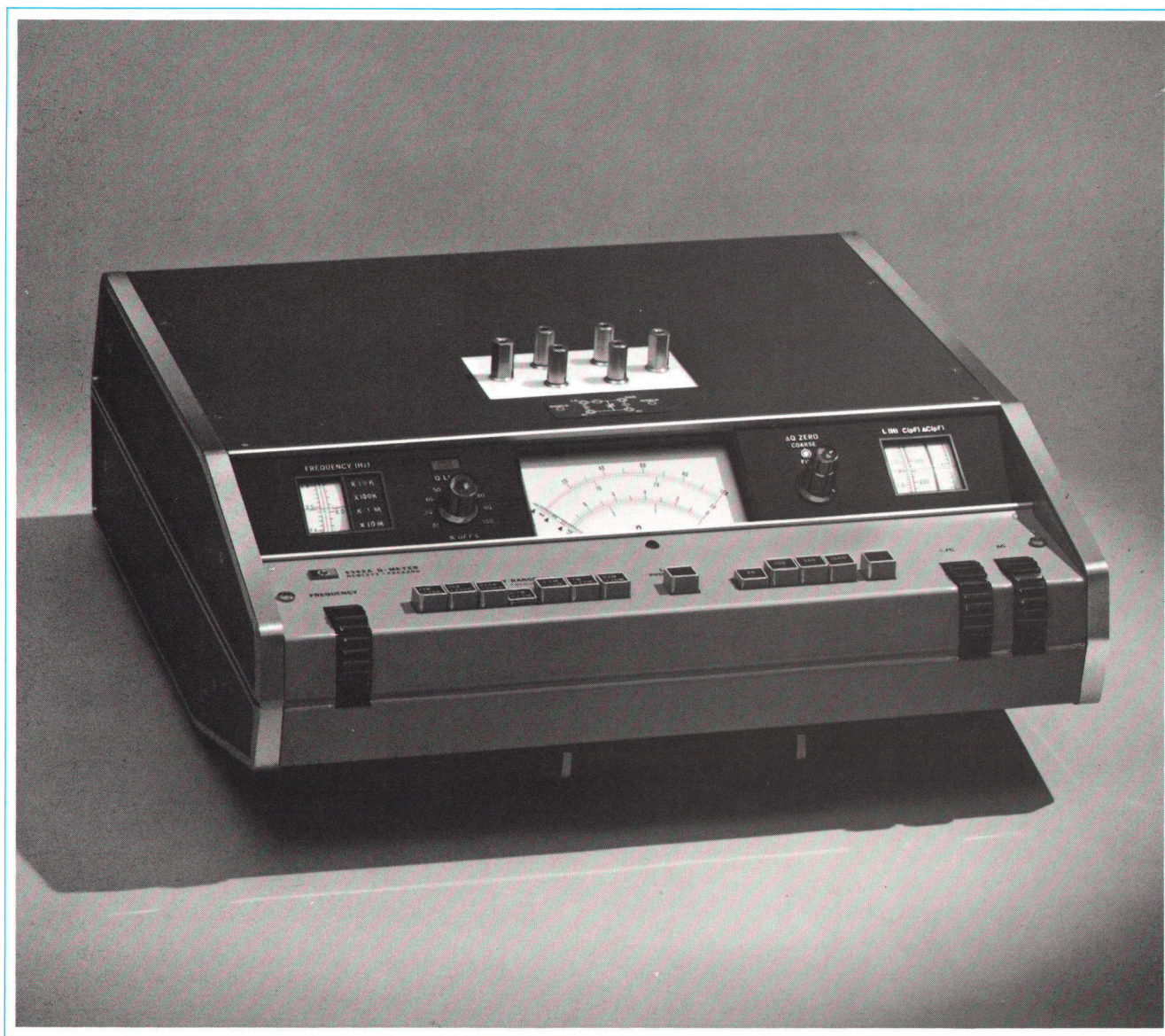
Fig. 2. Pushbutton controls simplify Q measurements with the new HP Model 4342A Q Meter. Q from 5 to 1000 can be measured in a frequency band from 22 kHz to 70 MHz.
