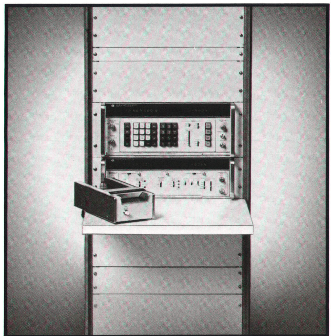
Fig. 4. Model 3041A Network Analyzer System has Marked Card Programmer for fast set-up and execution of tests.
