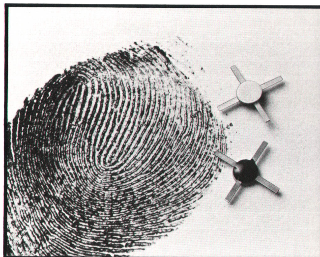
Fig. 9. Completed diode quad can be installed in circuits by conventional soldering techniques.
