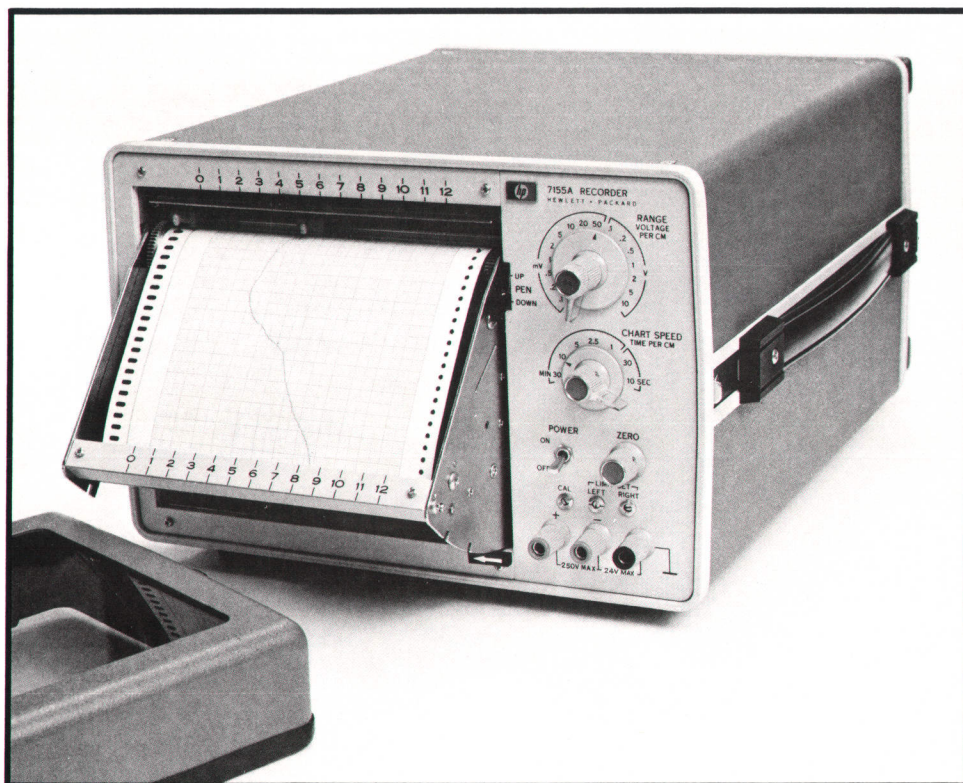
Fig. 1. Model 7155A Portable Strip-Chart Recorder is designed to deliver laboratory accuracy in field use. Pen displacement is accurate within \pm 0.5\% and chart speed is accurate within \pm 1\% , independent of ac line frequency, over a wide range of environmental conditions. Internal batteries are optional.
