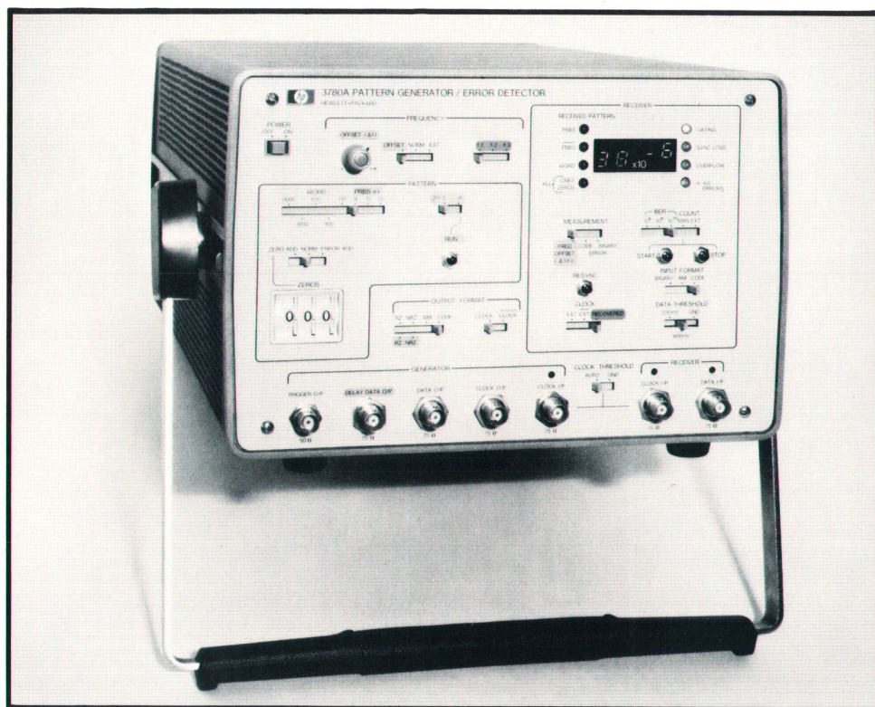
Fig. 1. Model 3780A Pattern Generator/Error Detector combines digital signal source and receiver in one portable package. A wide choice of output formats and automatic receiver synchronization facilitate its use on PCM communications systems.
