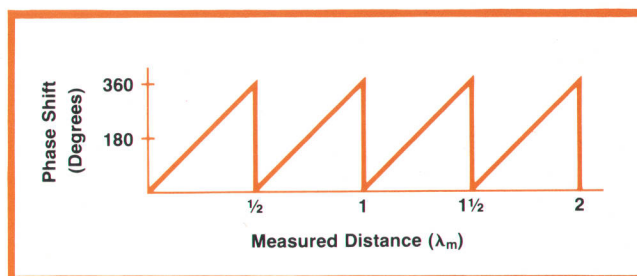
Fig. 4. Phase shift is a linear function of distance within one-half wavelength of the light-beam modulation signal. Two modulation frequencies are used: 75 kHz for the basic 2000-m measurement interval and 15 MHz for a 10-m interval and better resolution.
