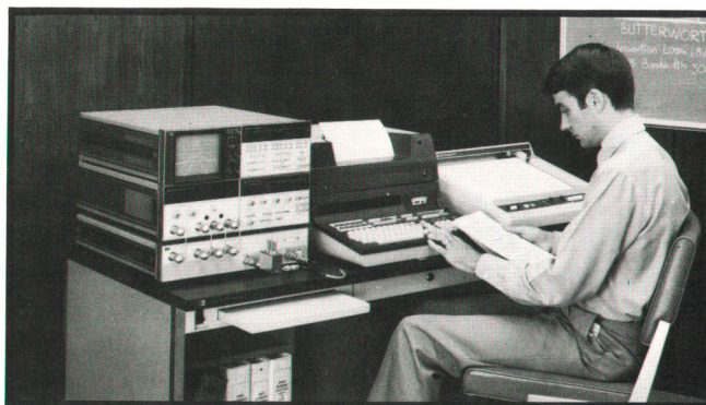
Fig. 5. Factory-assembled and tested automatic systems designed around the Model 8505A Network Analyzer are furnished with example programs and programs for accuracy enhancement, system verification, and diagnostic testing.
