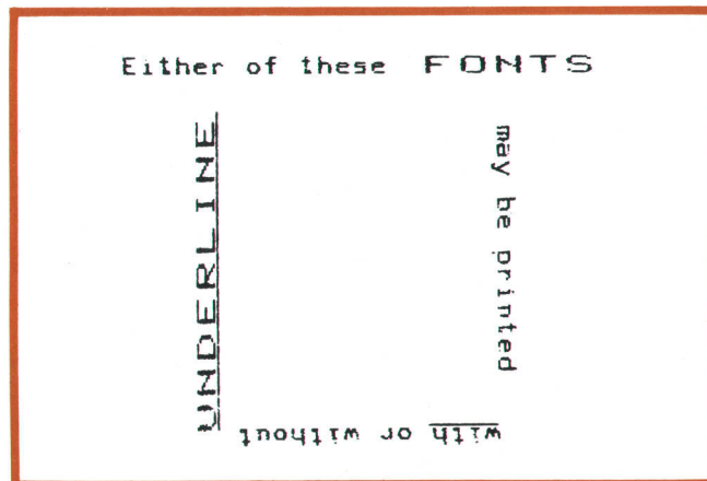
Fig. 3. For fast plot labeling, the plotter/printer can print dot matrix characters in four orthogonal directions.
