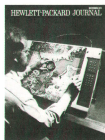
Cover: Model 9874A Digitizer transmits coordinate data to an on-line computer. Its tiltable, translucent platen adapts to a variety of media, including backlighted and rear-projected images. An EXTEND mode is provided for digitizing media larger than the platen. (Aerial photo courtesy of the U.S.A. National Aeronautics and Space Administration).
