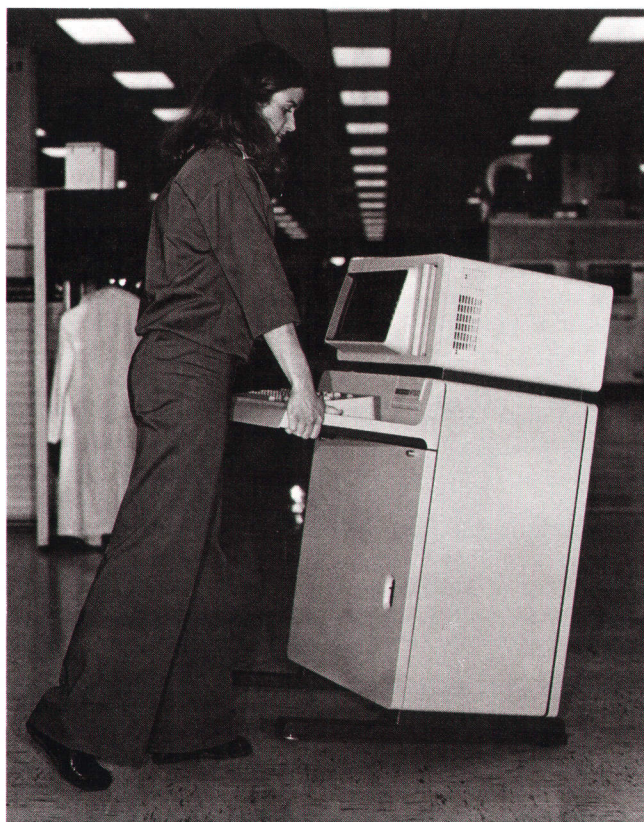
Fig. 4. HP 300 can be moved like a wheelbarrow.
