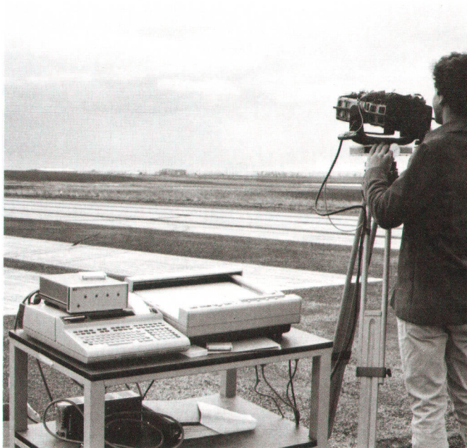
Fig. 13. Equipment used to measure the velocity of an airplane. The 3850A was an experimental model modified to produce an audible tone when pointed at the retroreflectors. The fixture holding the 3850A was also a special experimental model. (a) Experimental dynamic monitoring system. (b) Mounting of retroreflectors on the aircraft's wing.
