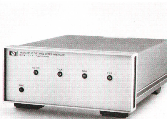
Fig. 1. Model 38001A Distance Meter HP-IB Interface makes four HP electronic distance meters compatible with the HP Interface Bus (IEEE 488-1978).
