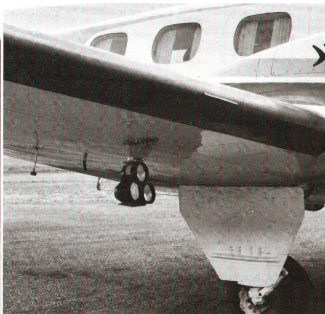
Fig. 13. Equipment used to measure the velocity of an airplane. The 3850A was an experimental model modified to produce an audible tone when pointed at the retroreflectors. The fixture holding the 3850A was also a special experimental model. (a) Experimental dynamic monitoring system. (b) Mounting of retroreflectors on the aircraft's wing.
