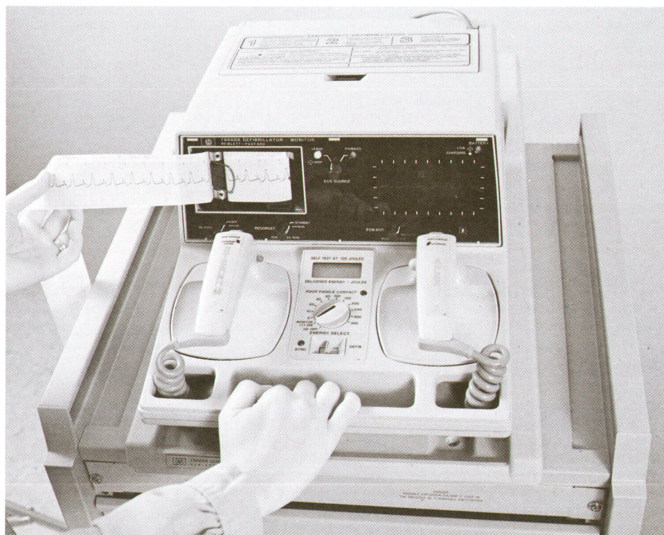
Fig. 1. The HP Model 78660A Defibrillator-Monitor is a convenient portable instrument for resuscitation, monitoring, and documentation in cardiac-arrest emergencies.
