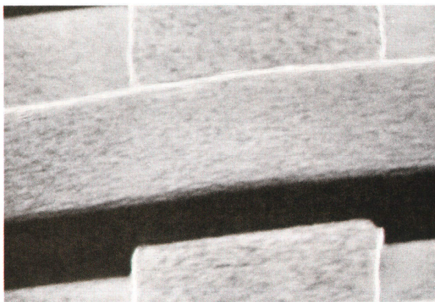
Fig. 1. Resist step coverage: 1- \mu\text{m} -thick resist pattern over 0.5- \mu\text{m} -high step.
