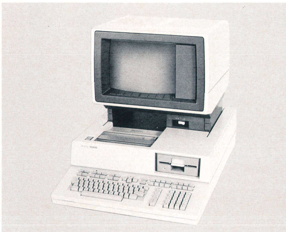
Fig. 1. The HP 9000 Model 520 Computer is a 32-bit computer system based on HP's NMOS-III VLSI and finstrate technologies. It provides professional personnel with a desktop workstation having mainframe computer capabilities. The Model 520 contains its own printer, hard and flexible disc memory devices, I/O processor, and keyboard. Several CRT display options are available. The Model 520 can have up to three CPUs for increased performance in computation-intensive applications or up to 2.5 megabytes of RAM for data-intensive work. For I/O-intensive work, up to three I/O processors can be installed.
