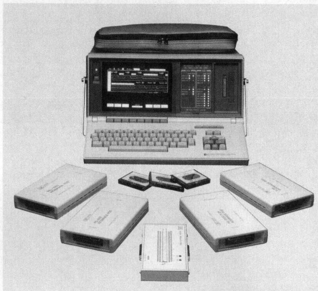
Fig. 3. The HP 4953A Protocol Analyzer connects to the network under test through a network-specific interface pod. It has a menu-driven softkey user interface and a built-in cartridge tape unit for reading and storing data and applications programs.
