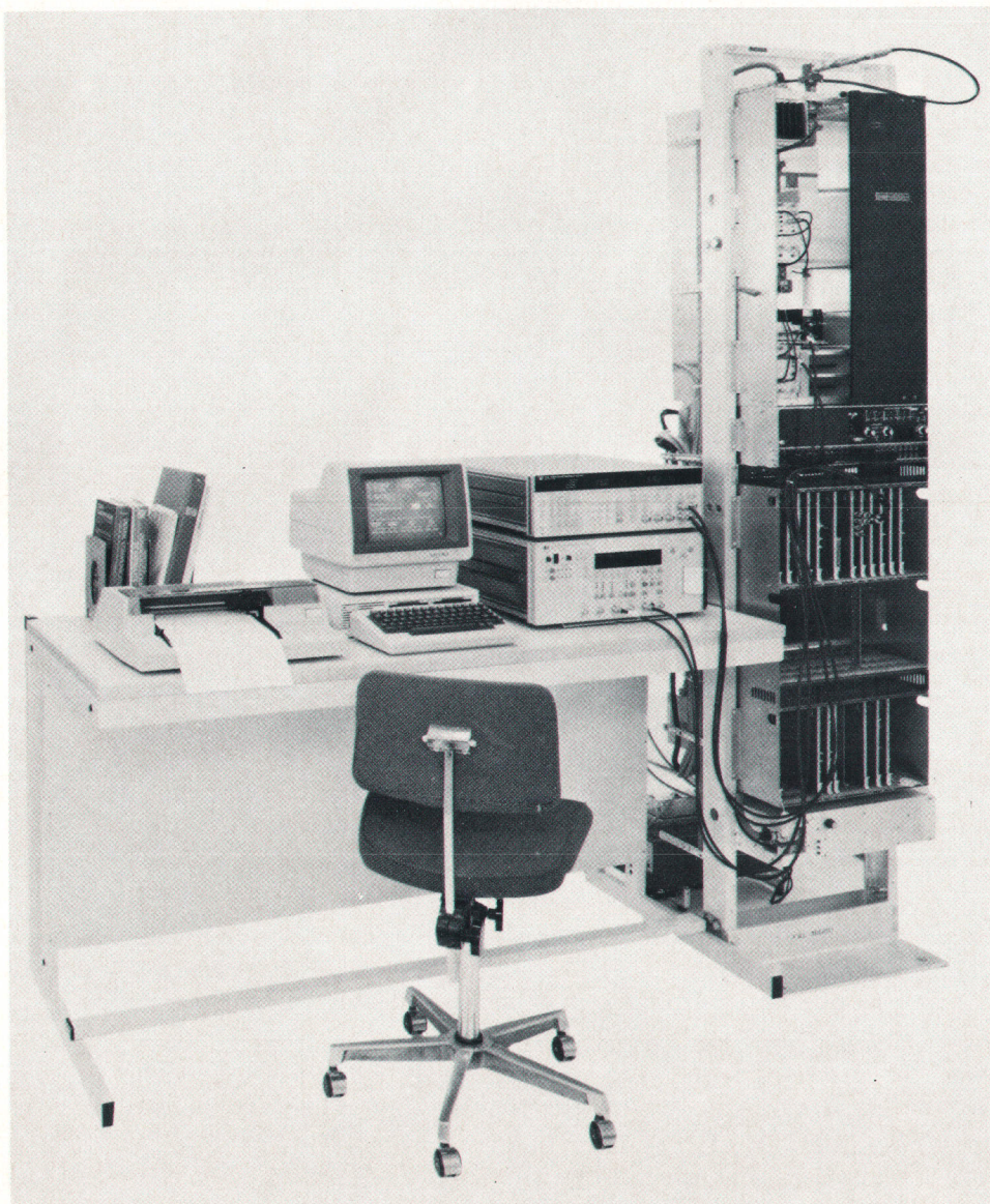
Fig. 2. HP 3708S Noise and Interference Measurement System.
