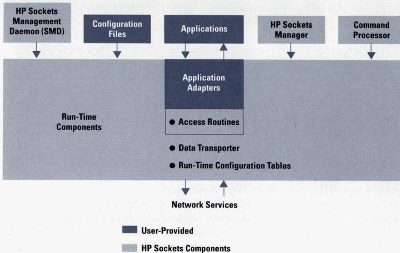
Fig. 2. HP Sockets run-time and administration components.
