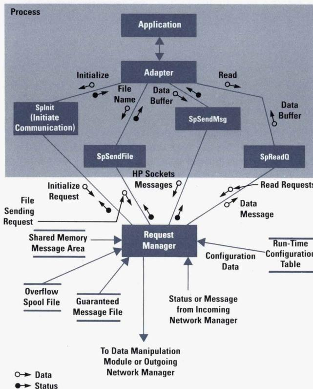
Fig. 7. Structure chart showing the communication data flows between the request manager and some of the HP Sockets access routines.
