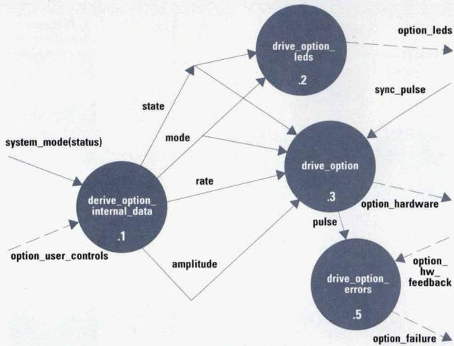
Fig. 4. Data flow diagram for example subsystem.
