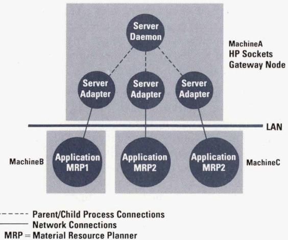
Fig. 1. A server daemon and three server adapters running on the gateway node (**MachineA**).
