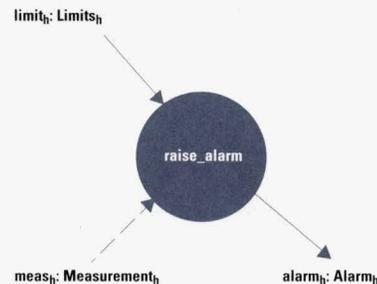
Fig. 6. Data flow diagram of the raise\_alarm process with the correct data flows.
