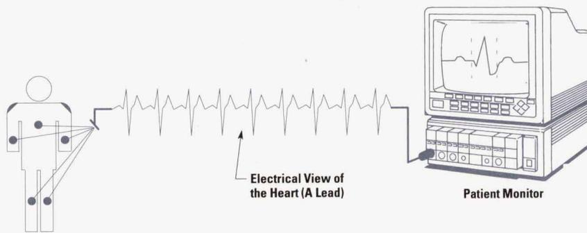
**Fig. 2.** Setup for making ECG measurements, showing the stream of voltage signals from one of the ECG leads.
