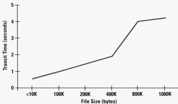
Fig. 2. HP Sockets file transit time as a function of file size using an HP 9000 Series 370.
