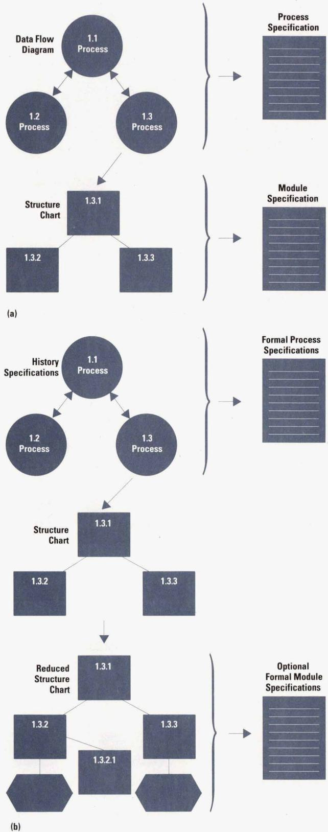
**Fig. 3.** The production of module specifications. (a) In the traditional SA/SD approach they are produced after structure charts are defined. (b). In the formal specification implementation, the process specification can usually replace the need for module specifications.
