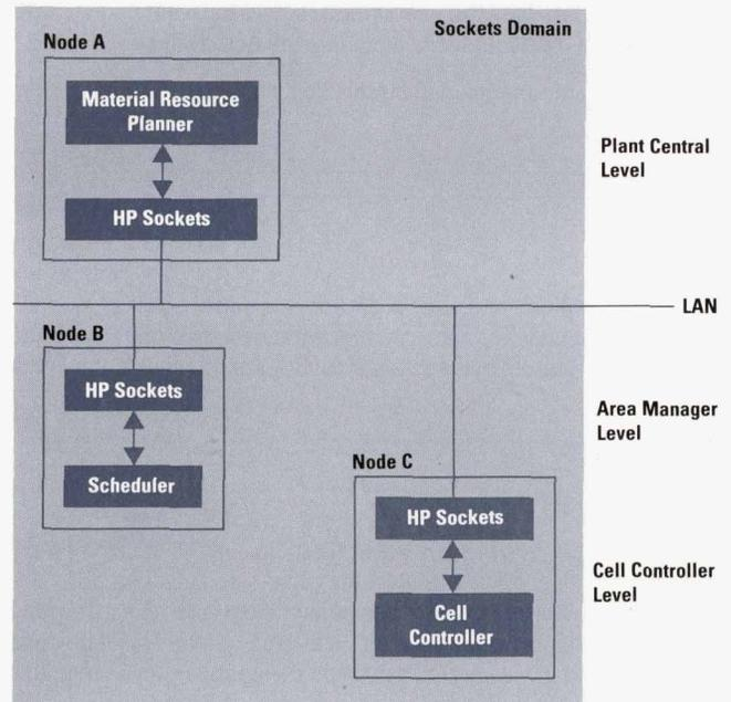
Fig. 1. Examples of the type of applications that might be integrated in the HP Sockets domain.
