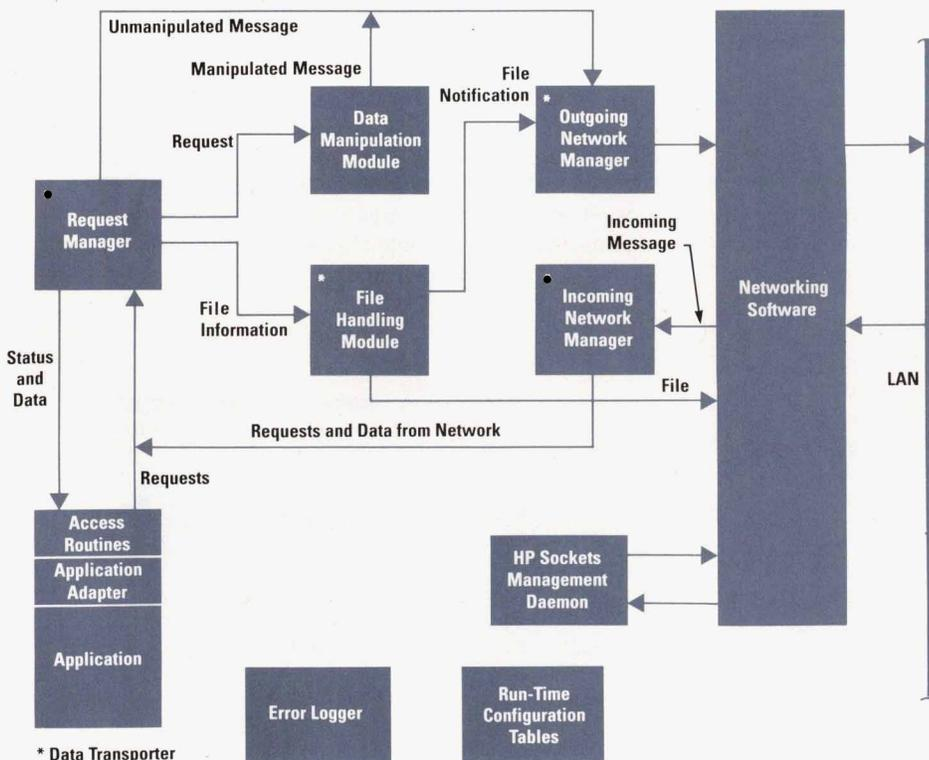
**Fig. 4.** HP Sockets run-time architecture.
