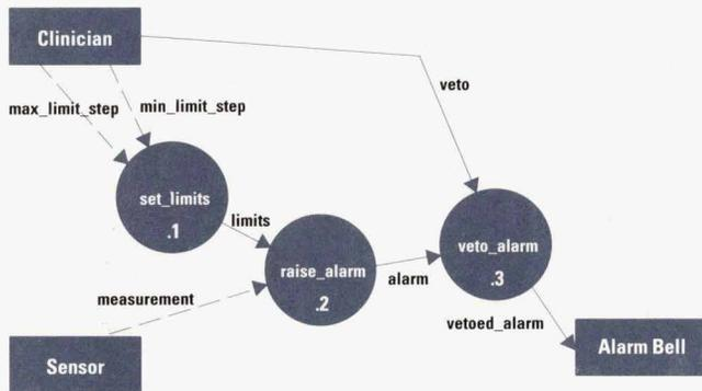
Fig. 1. Composition diagram for the alarm system.
