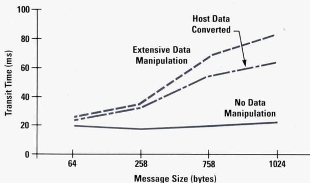
Fig. 3. HP Sockets message transit time as a function of message size using two HP 9000 Series 370s.
