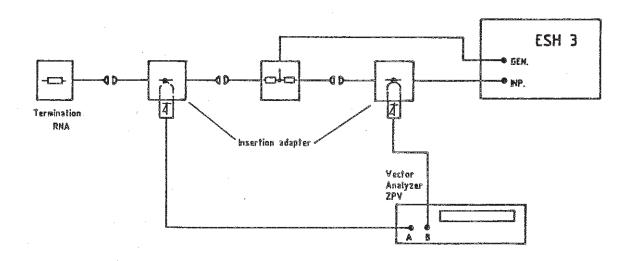
The reflection-coefficient indicator, such as the ZPV, operates at the frequency to which the receiver is tuned.
