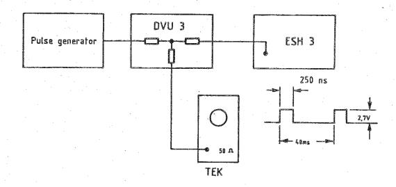
The pulse generator (pulse repetition frequency 25 Hz) supplies the standard pulse required in compliance with CISPR 3 (EMF 1.35  $\mu$ Vs = 5.4 V · 250 ns;  $Z_{\rm out}$  = 50  $\Omega$ )
