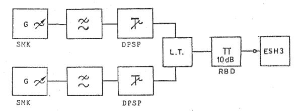
Both signal generators are set to maximum output. The attenuation of the lowpass filters must be > 60 dB at twice the wanted signal.
