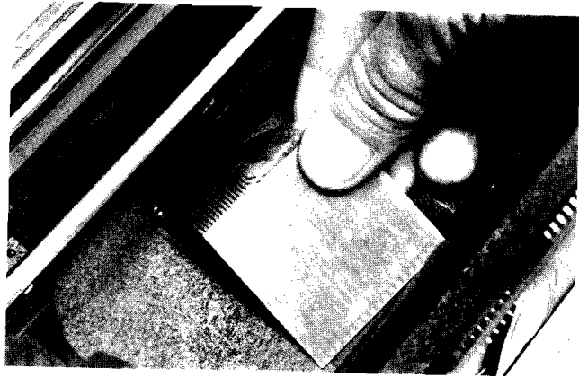
Figure 4-3. Removing Print Head Flex Cable Connector
