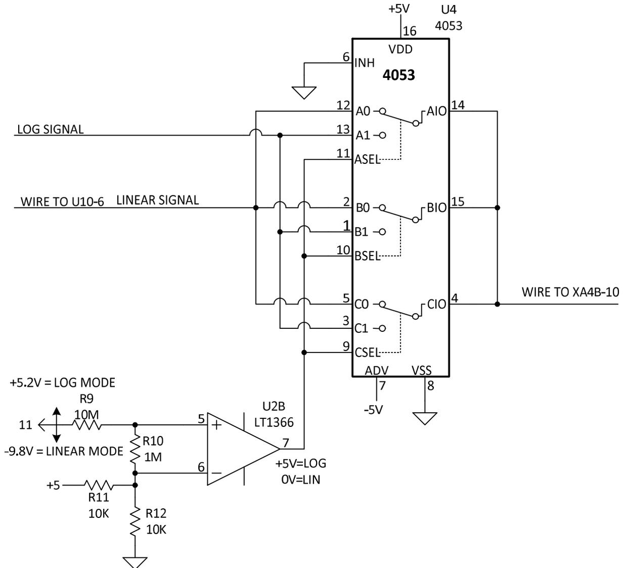
Figure 4b: Part 2 of schematic diagram of new log amplifier
