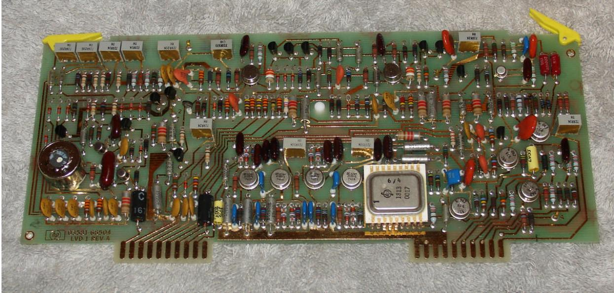
Figure 1: Picture of HP3580A A4 Detector Board
