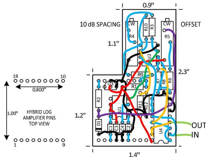
Figure 5: Component location and wiring of new log amplifier (top view)
