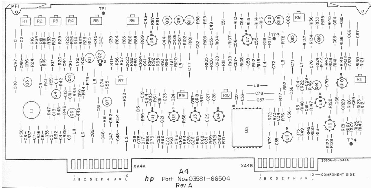
Figure 3: Board layout of 3580A A4 Detector board
