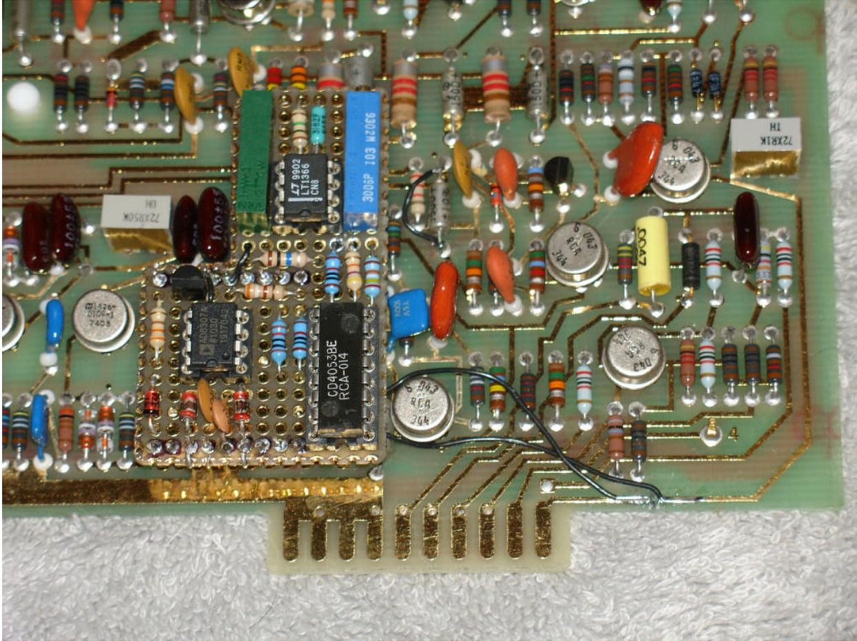
Figure 7: New log amplifier installed
