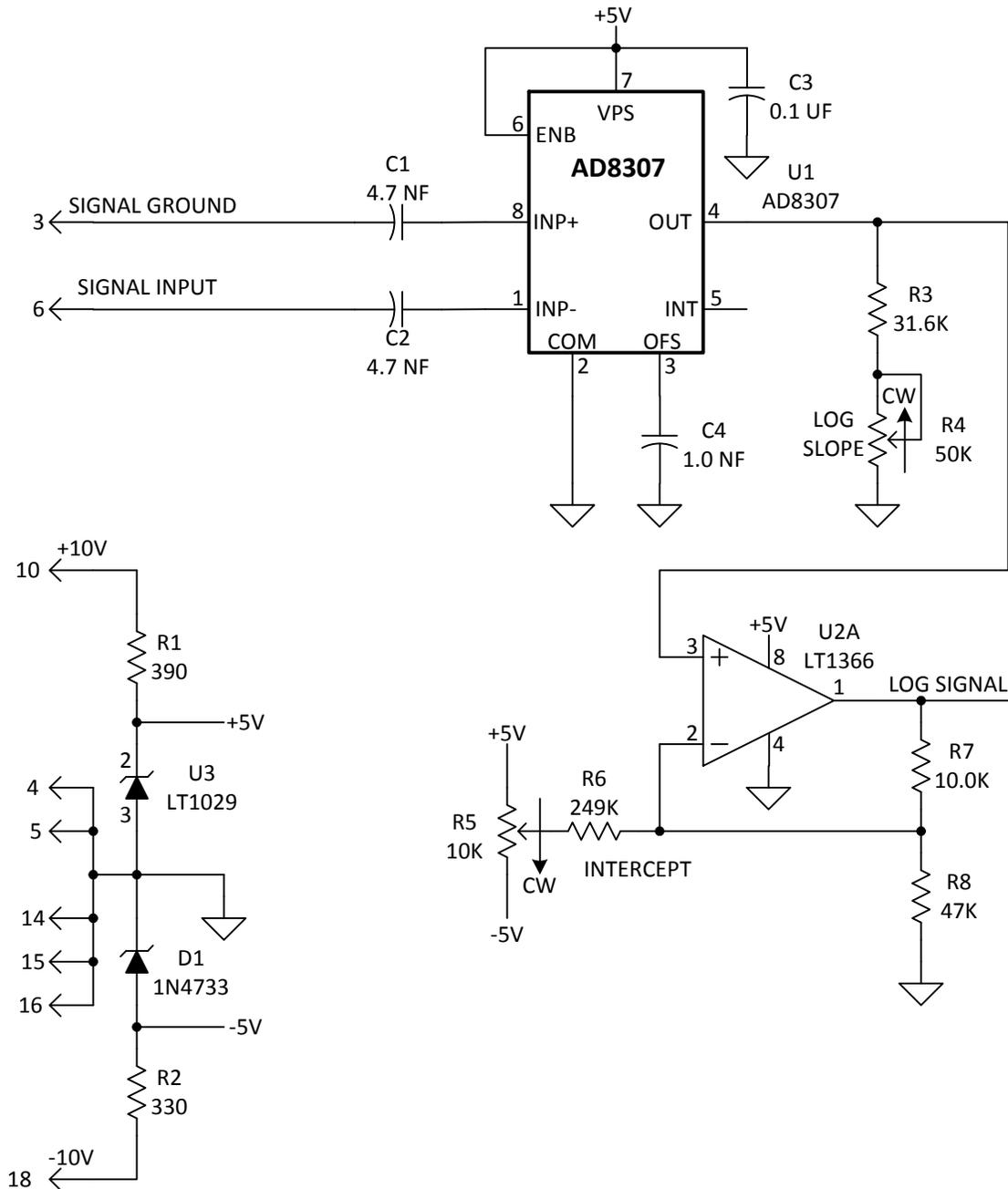
Figure 4a: Part 1 of schematic diagram of new log amplifier
