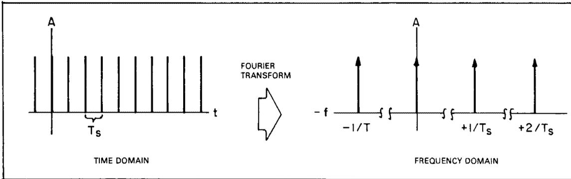
**Figure 3-31. Frequency Representation of an Impulse Train.**
