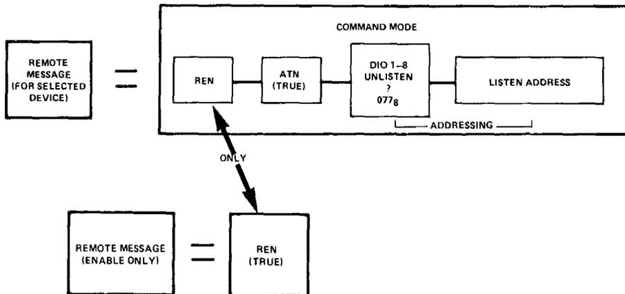
**LOCAL** – The Local Message will remote addressed instruments from remote Operation mode to Local-Front panel control. The controller must place the HP-IB into the command Mode and address all instruments to listen that are to be returned to local. The local message will not remove the bus from the remote mode, only the listening devices.
