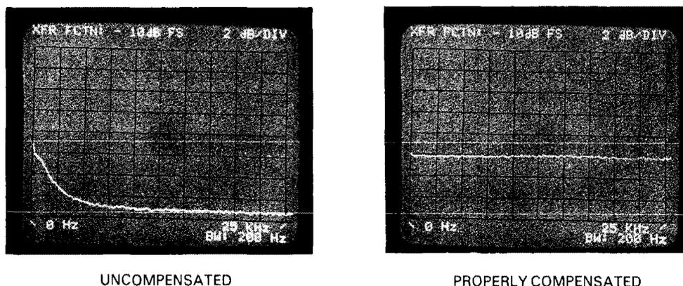
**Figure 3-26. Probe Compensation.**
