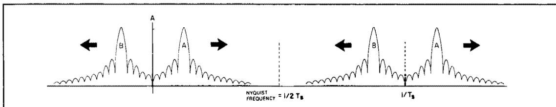
**Figure 3-35. Increasing the Frequency of a Cosine Wave.**
