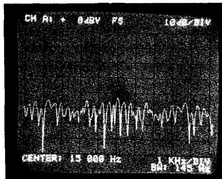
**Figure 3-18. Modulating a Spectral Line with Noise.**
