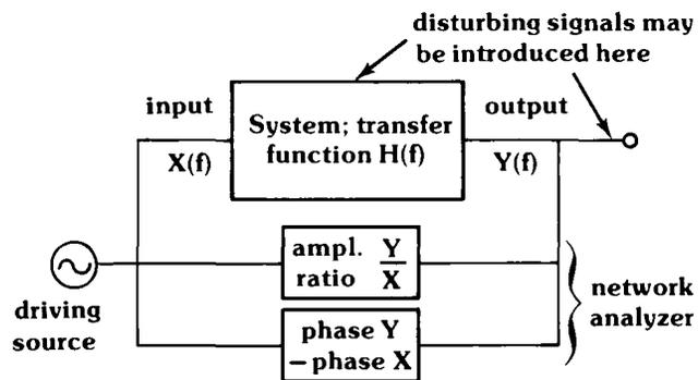
It is evident that determining the transfer function  $H(f)$  by calculating the spectral ratio  $Y(f)/X(f)$  will lead to irrecoverable errors whenever there is a disturbing signal included with the output  $Y(f)$ . The 3582A reduces these errors through a computational technique: it uses the cross power spectrum (see appendix) and spectrum averaging. The question remains, however, how many averages are needed to attain a desired accuracy?
