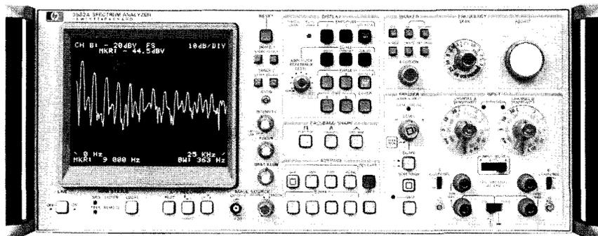
The HP 3582A is a spectrum analyzer covering the frequency range of DC to 25 kHz. Although it is a FFT-based, digital instrument, a special design effort has made it as straightforward to use as a conventional swept analyzer. With dual measurement channels it is possible to measure transfer function gain and phase, as well as the coherence function. A built-in random or pseudo-
