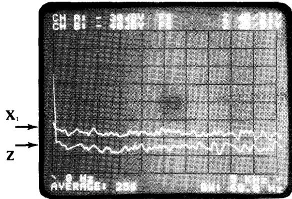
b) Measured filter transfer functions.
