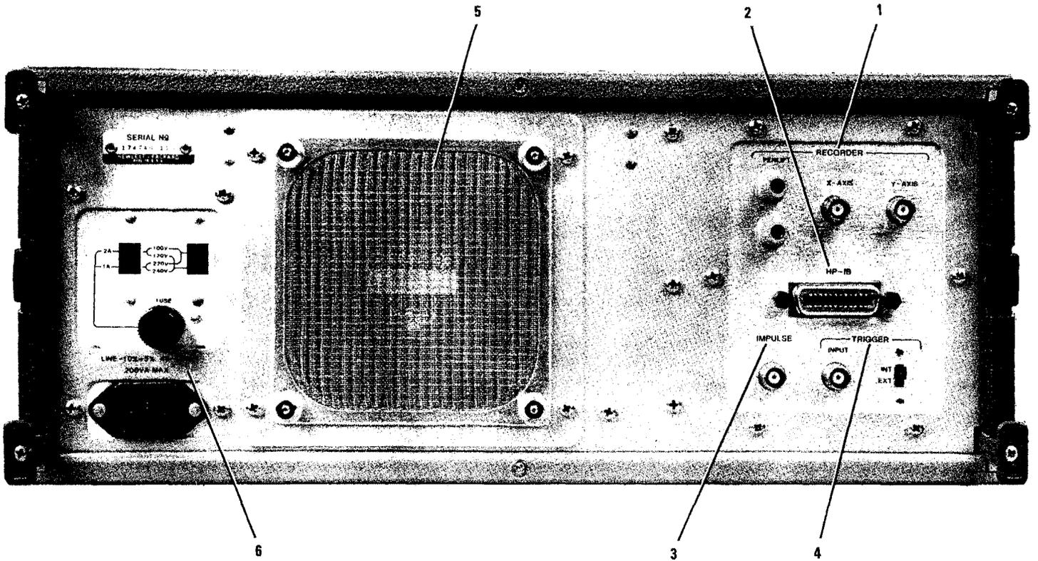
Figure 3-49. 3582 Rear Panel Connectors, Switches, and Filter.
