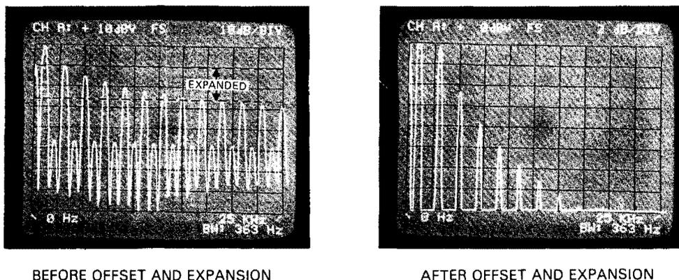
**Figure 3-5. Expanding a Portion of the Display.**
