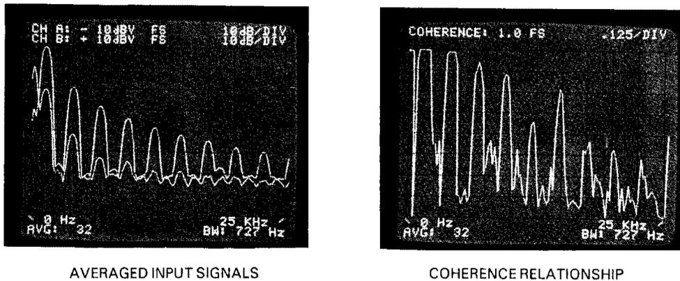
**Figure 3-23. The Coherence Relationship Between Two Signals.**
