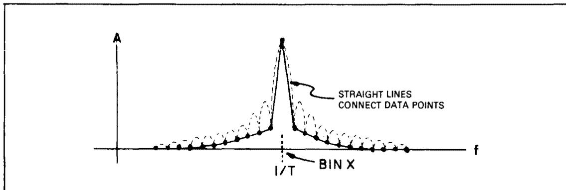
**Figure 3-40. Memory Data Points Displayed on CRT.**
