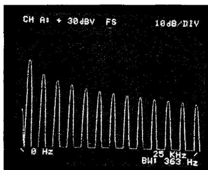
**Figure 3-2. Spectrum of a 1 kHz Square Wave.**
