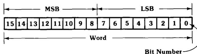
**2's COMPLEMENT.** A means of representing both positive and negative integers with binary numbers. In the 3582A, fundamental processing and storage occurs with 16 bit, 2's complement words, spanning a numeric range of -32768 to +32767. See page 43 of "Understanding the HP 3582A Spectrum Analyzer."
