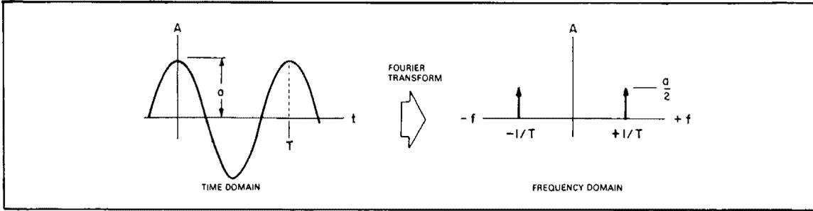
**Figure 3-30. Frequency Representation of a Cosine Wave.**
