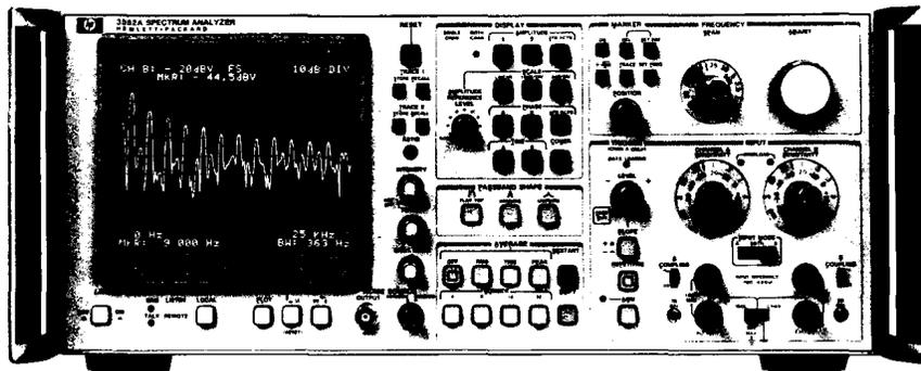
The HP 3582A is a spectrum analyzer covering the frequency range of DC to 25 kHz. Although it is a FFT-based, digital instrument, a special design effort has made it as straightforward to use as a conventional swept analyzer. With dual measurement channels it is possible to measure transfer function gain and phase, as well as the coherence function. A built-in random or pseudo-
