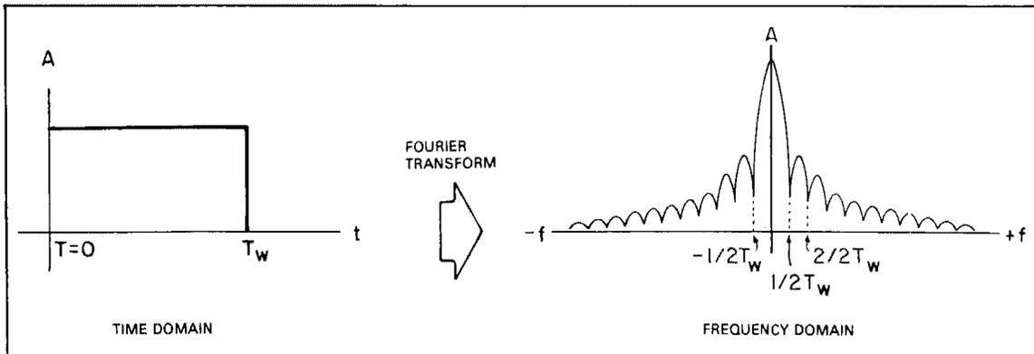
**Figure 3-32. Frequency Representation of a Square Pulse.**
