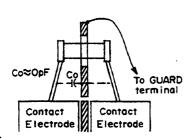
To reduce such stray capacitances, insert the component leads deeply into the test fixture. Measurement accuracy for low capacitance sample can be improved by using a guard to eliminate the stray capacitances. Place guard plate between component leads of the sample and connect it to instrument GUARD terminal as illustrated at left:
