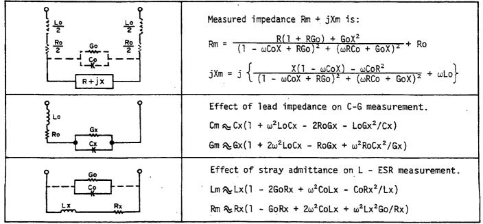
Figure 3-9. Residuals Present in Measuring Circuit.
