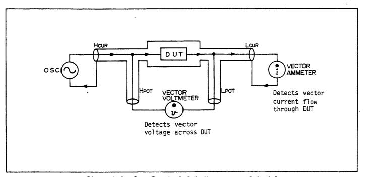
Figure 3-6. Four Terminal Pair Measurement Principle.
