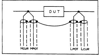
Figure 3-5. Four Terminal Pair DUT Connections.
