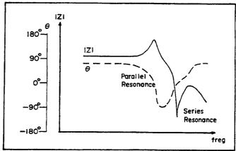
Figure 3-11. Effect of Resonance in sample (example).
