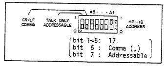
Figure 3-23. HP-IB Control Switch.
