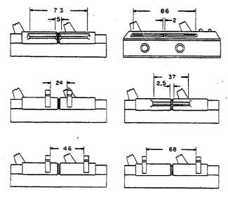
Dimensions of Test Fixture Contacts. (Unit = mm)
