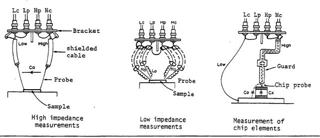
Figure 3-18. Semiconductor Device Measurement (sheet 3 of 3).
