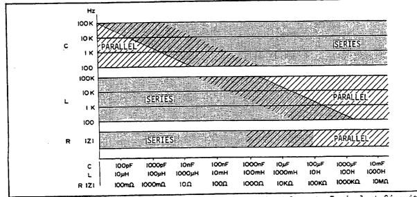
Figure 3-4. Approximate Relationships of Sample Values to Equivalent Circuit.
