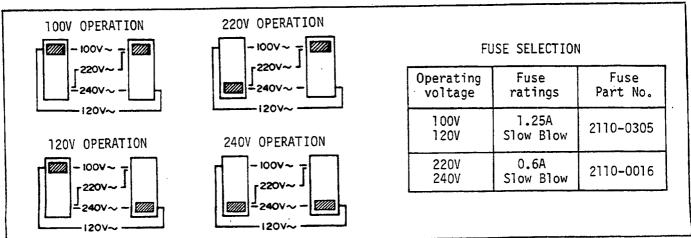
Figure 2-1. Line Voltage and Fuse Selection.
