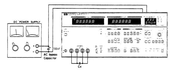
To make capacitance measurements using external dc bias voltages up to  $\pm 200$ V, connect dc bias source and test fixture as shown in diagram. If maximum applied dc bias voltage exceeds  $\pm 35$ V, use operating PROCEDURE A. If not, use PROCEDURE B to obtain a shorter bias voltage settling time.
