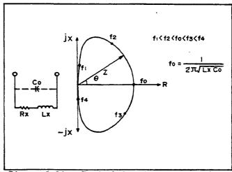
Figure 3-13. Typical Impedance Locus of an Inductor.
