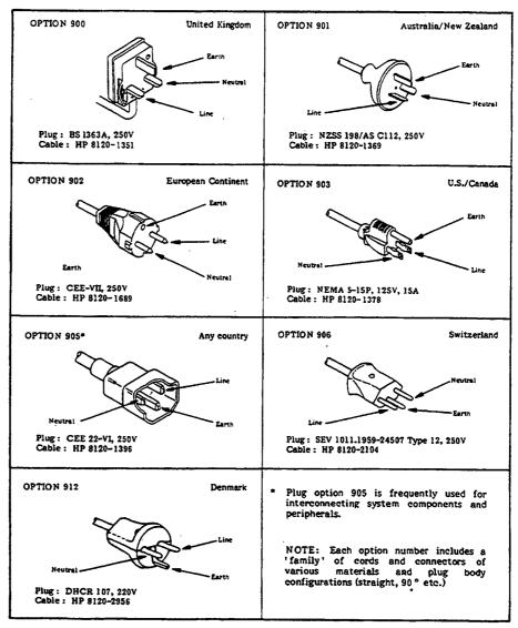
Figure 2-2. Power Cables Supplied
