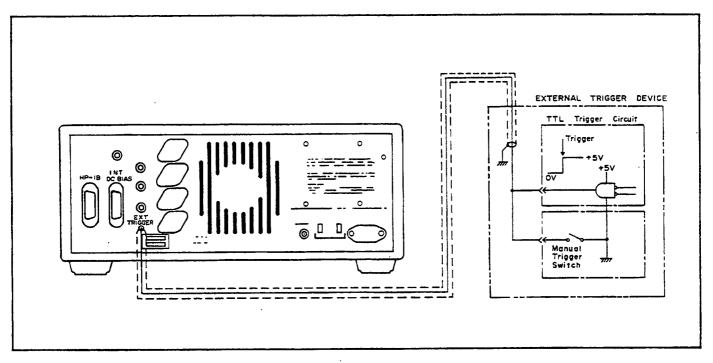
Figure 3-15. External Trigger Circuit.
