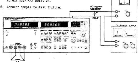
Figure 3-19. External DC Bias Circuits (sheet 4 of 4).
