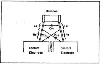
Figure 3-10. Parasitic Impedances
