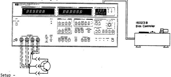
The figure above is a typical test setup used for measuring the base-collector junction capacitance (Cob) of an NPN transistor. For this measurement, the appropriate test fixture may be user designed. A 4274A unit equipped with option 001 (or option 002) is suitable for controlling the accurate dc bias required for the measurement. If dc bias is not necessary, setup arrangement and procedures associated with this measurement may be deleted.
