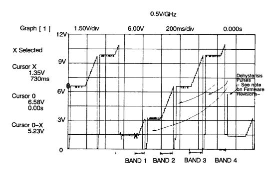
Figure 12-3. Rear-Panel SWP Output
