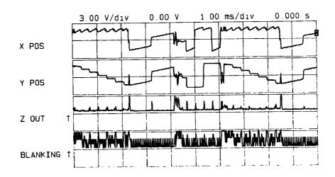
Figure 10-2. Line Generator Output Waveforms
