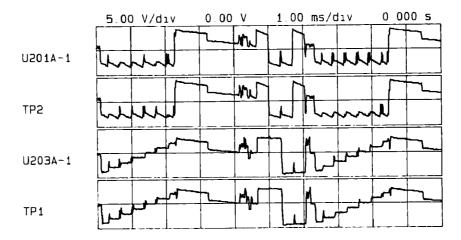
Figure 10-6. Distorted X/Y Line Generator Waveforms
