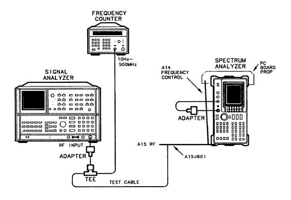
Figure 2-19. Signal ID Oscillator Adjustment Setup
