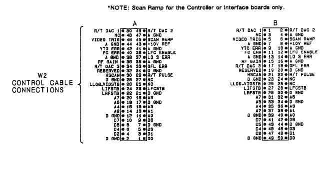
Figure 7-2 Ribbon Cable Connections (1 of 2)
