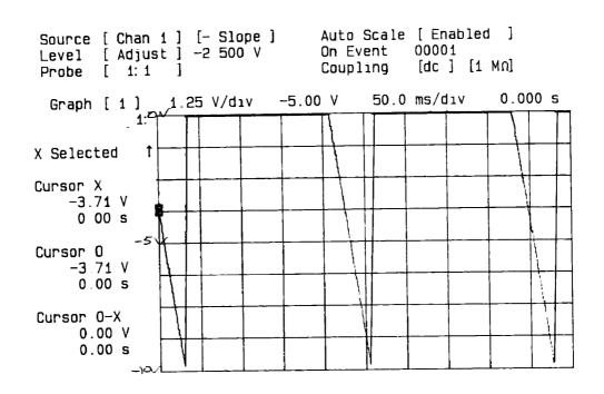
Figure 11-7. Input to Main/FM/VCO Sweep Switch
