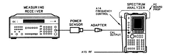
Figure 2-13. Calibrator Amplitude Adjustment Setup
