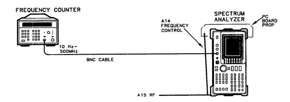
Figure 2-14. 10 MHz Frequency Reference Adjustment Setup
