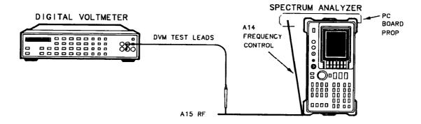
Figure 2-6. Sampler Adjustment Setup
