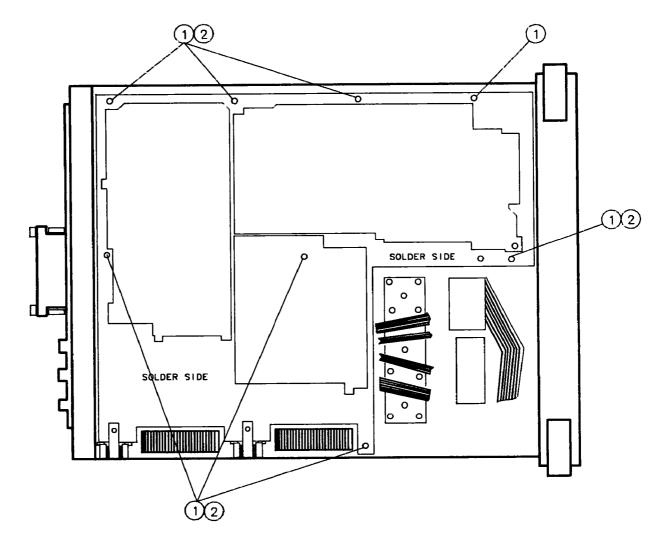
Figure 3-21. A14 and A15 Assembly Removal
