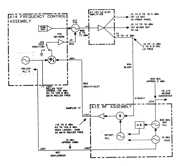
Figure 11-12. Simplified Synthesizer Section
