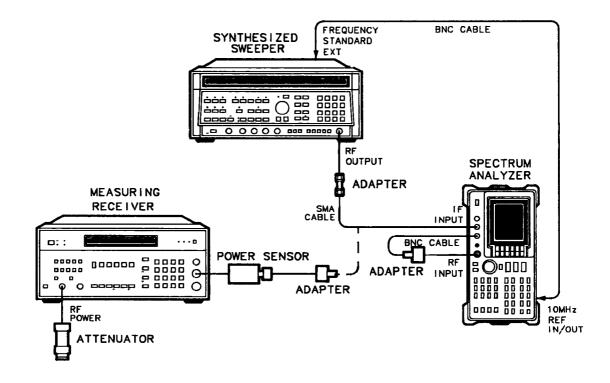
Figure 2-17. External Mixer Amplitude Adjustment Setup
