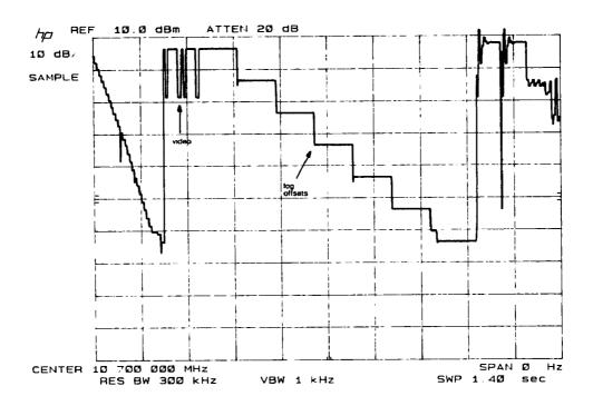
Figure 9-7. Detailed IF Adjust Signature (4)
