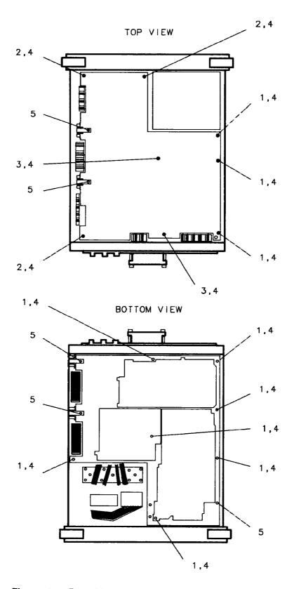
Figure 4-1. Parts Identification, Assembly Mounting (1 of 2)
