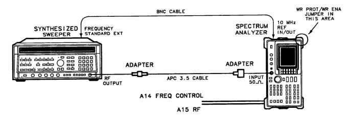
Figure 2-11. YTF Adjustment Setup
