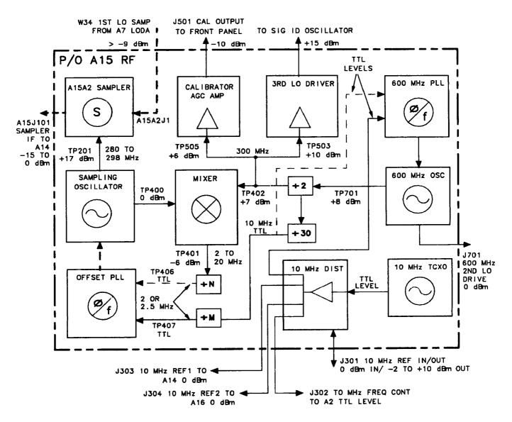
Figure 11-14. Simplified A15 Assembly Block Diagram
