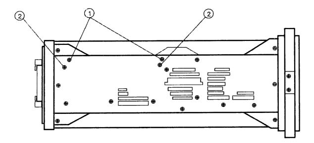
Figure 3-14. A17 CRT Driver Mounting Screws
