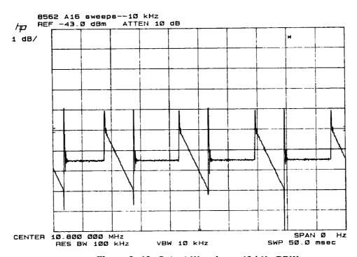
Figure 9-16. Output Waveform, 10 kHz RBW
