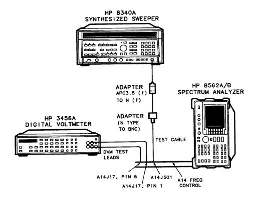
Figure 11-1. YTO Loop Test Setup
