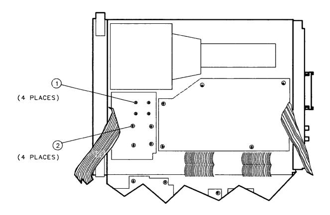
Figure 3-19. A10 Mounting Screws
