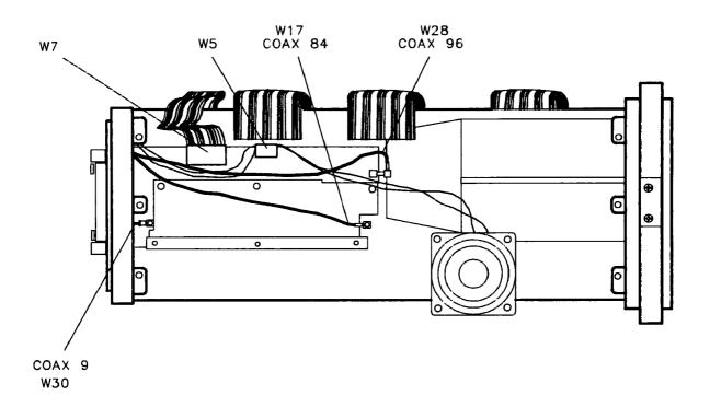
Figure 3-15. A16 Cable Routing
