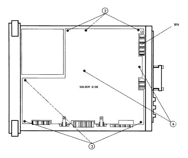
Figure 3-8. A2, A3, A4, and A5 Assembly Removal
