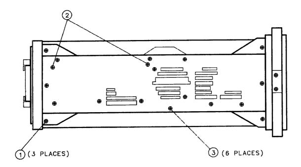
Figure 3-30. Side Frame Mounting Screws
