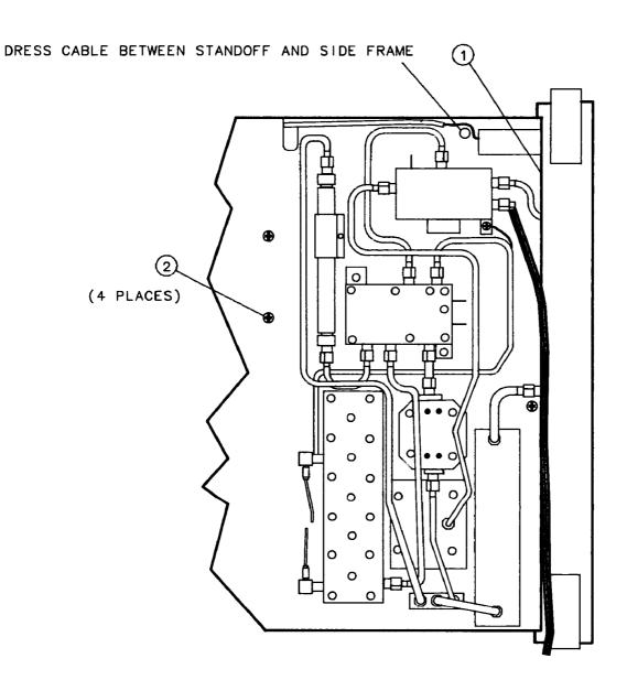
Figure 3-28. Line Switch Mounting Screw and Cable Dress
