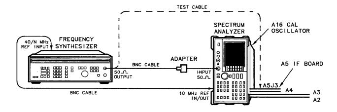
Figure 2-5. IF Amplitude Adjustment Setup
