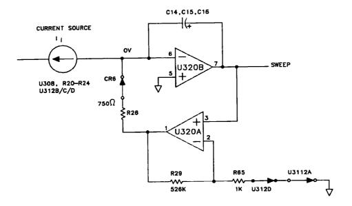
Figure 11-11. Simplified Sweep Generator during Retrace
