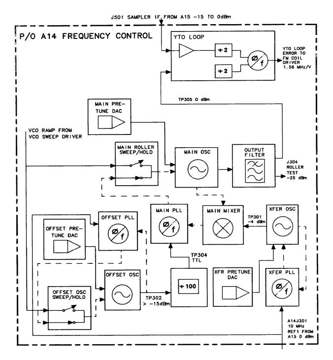
Figure 11-13. Simplified A14 Assembly Block Diagram
