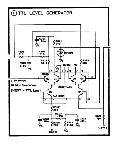
Figure 6-7. P/O A15 Schematic, (Manual Change 8)
