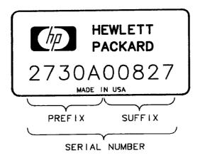
Figure 1-1. Typical Serial Number Label
