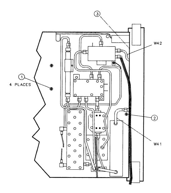
Figure 3-3. A9, A18, and Line-Switch Assembly Mounting Screws
