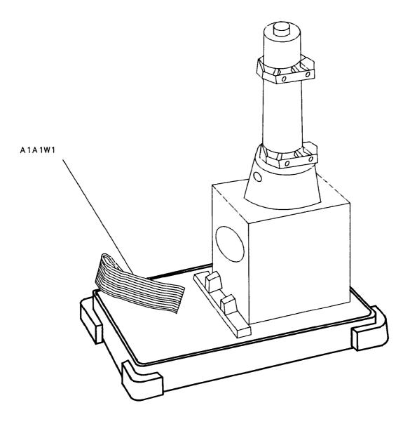
Figure 3-6. Placing the CRT into the Front Frame
