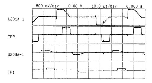
Figure 10-8. Normal X/Y Line Generator Waveforms
