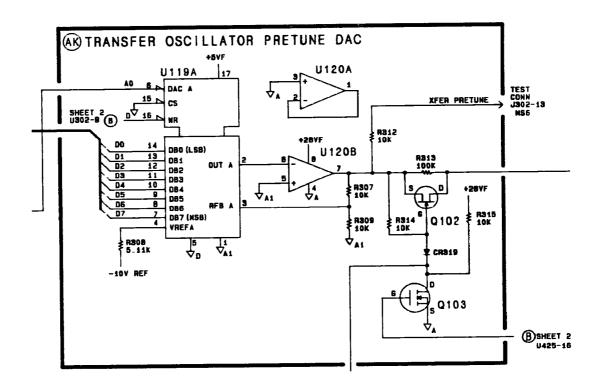
Figure 6-2. P/O A14 Schematic, AK (Manual Change 6)
