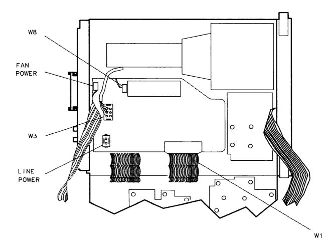
Figure 3-12. A6 Power Supply Connections
