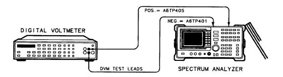
Figure 2-1. High Voltage Power Supply Adjustment Setup
