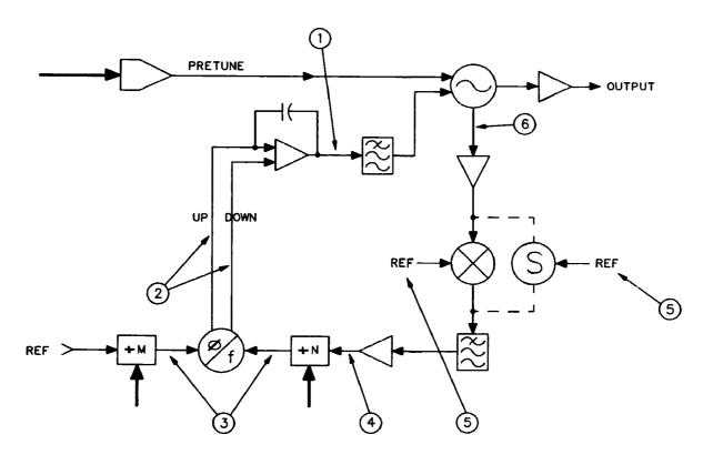
Figure 11-5. Unlocked PLL
