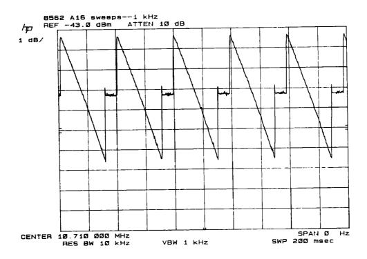
Figure 9-18. Output Waveform, 1 kHz RBW
