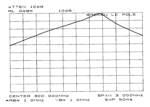
Figure 9-14. Faulty LC Pole
