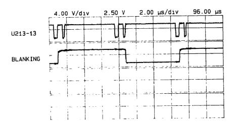
Figure 10-4. Expanded Blanking Waveforms
