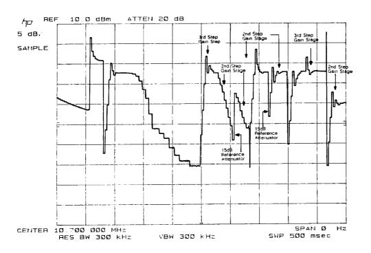
Figure 9-5. Detailed IF Adjust Signature (2)
