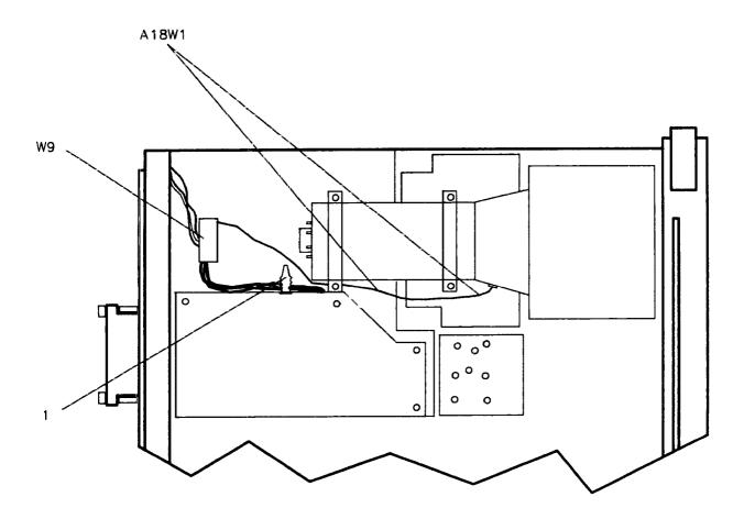
Figure 3-5. Installing the CRT and Front-Frame Assemblies
