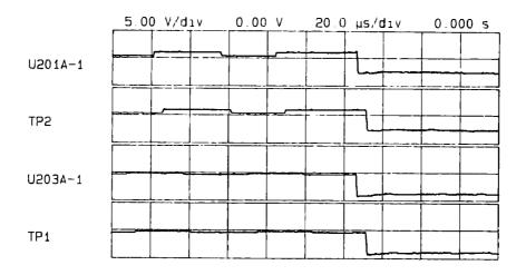
Figure 10-7. Expanded X/Y Line Generator Waveforms
