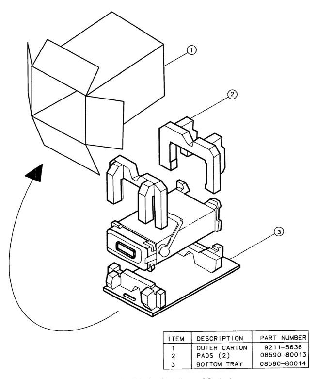
Figure 1-3. HP 8562A/B Shipping Container and Contents
