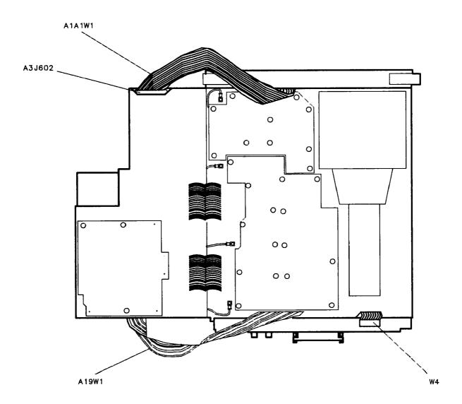
Figure 3-11. HP-IB and A1A1 W1 Cable Placement
