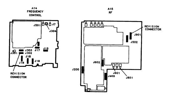
Figure 12-1. A14 and A15 Test Connectors
