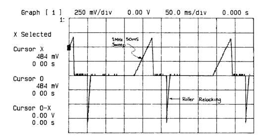
Figure 11-6. Input to YTO FM Coil Driver
