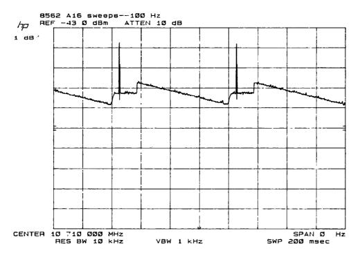
Figure 9-20. Failed Crystal Set Symptoms
