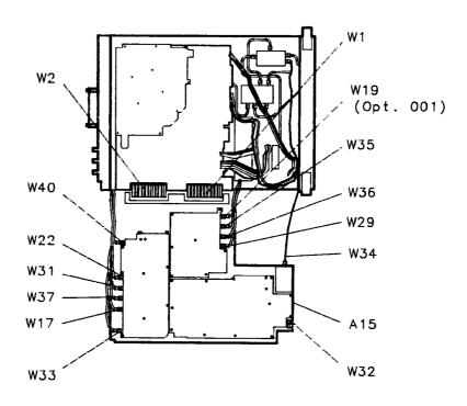
Figure 5-5. Bottom View (A15 Unfolded)
