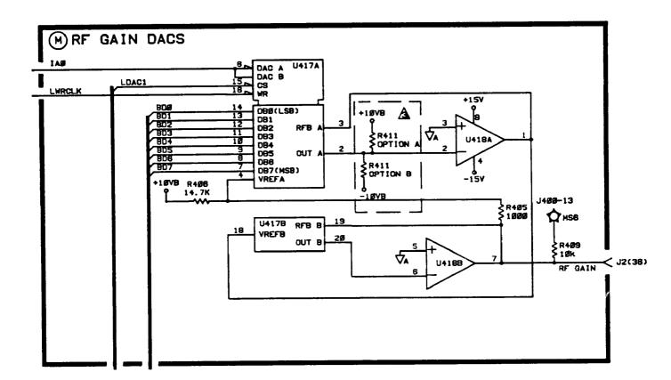
Figure 6-4. P/O A3 Schematic, M (Manual Change 7)
