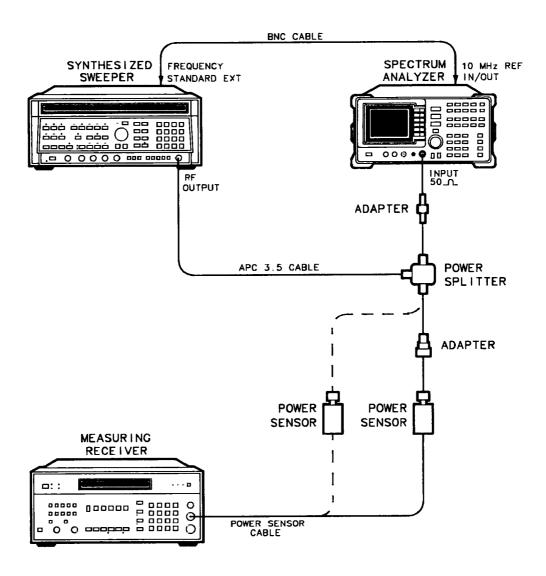
Figure 2-12. Frequency Response Adjustment Setup
