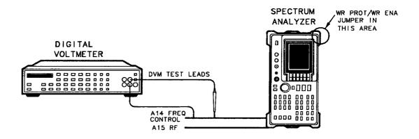
Figure 2-10. Dual Band Mixer Bias Adjustment Setup
