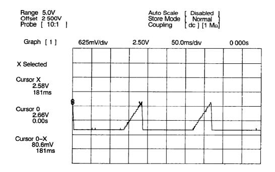
Figure 12-4. Signal at A14J15 Pin 1
