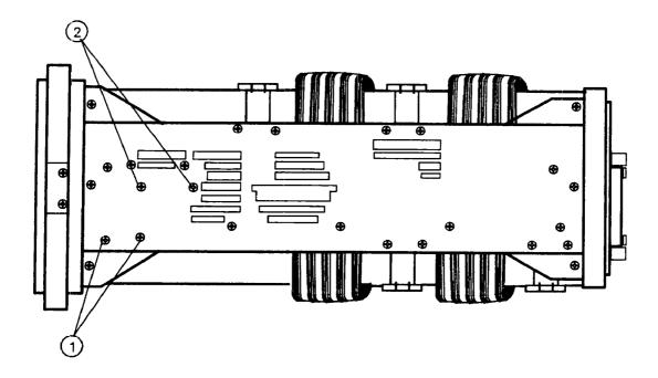
Figure 3-18. A9 Mounting Screws at Right Frame
