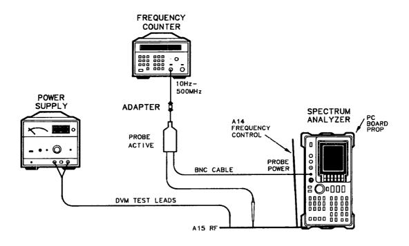
Figure 2-7. Coarse-Tune Adjustment Setup
