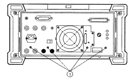
Figure 3-25. Main Deck Screws
