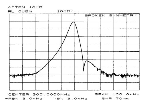
Figure 9-15. Faulty Crystal Symmetry
