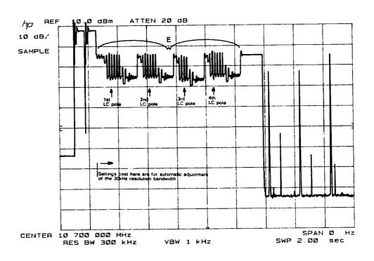
Figure 9-8. Detailed IF Adjust Signature (5)
