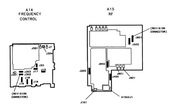
Figure 11-3. A14 and A15 Test Connectors
