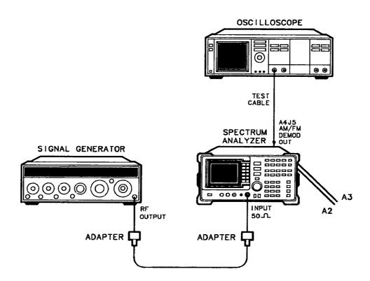
Figure 2-15. Demodulator Adjustment Setup
