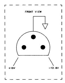
Figure 13-3. Probe Power Socket
