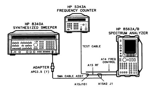
Figure 11-2. Sampler and Sampling Oscillator Test Setup
