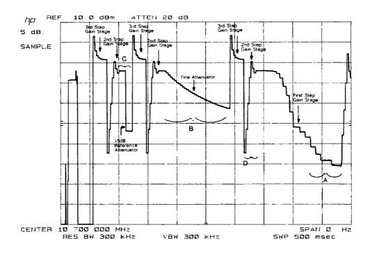
Figure 9-4. Detailed IF Adjust Signature (1)
