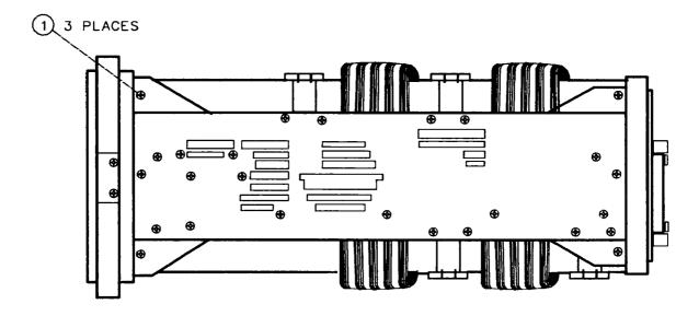
Figure 3-4. Front-Frame Mounting Screws
