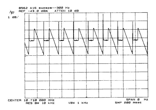
Figure 9-19. Output Waveform, 300 Hz RBW
