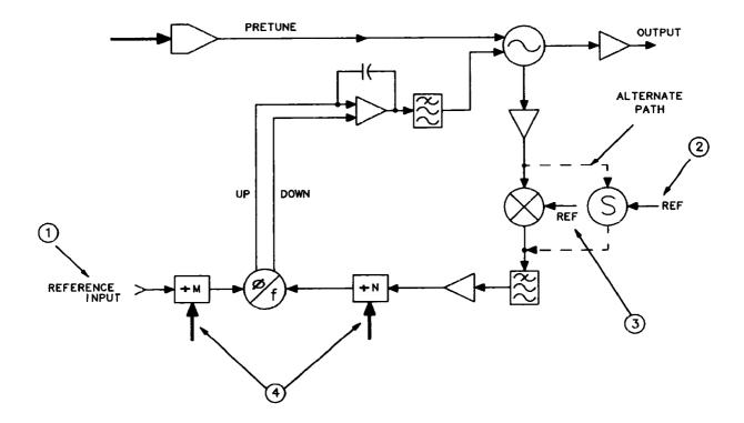
Figure 11-4. PLL Locked at Wrong Frequency
