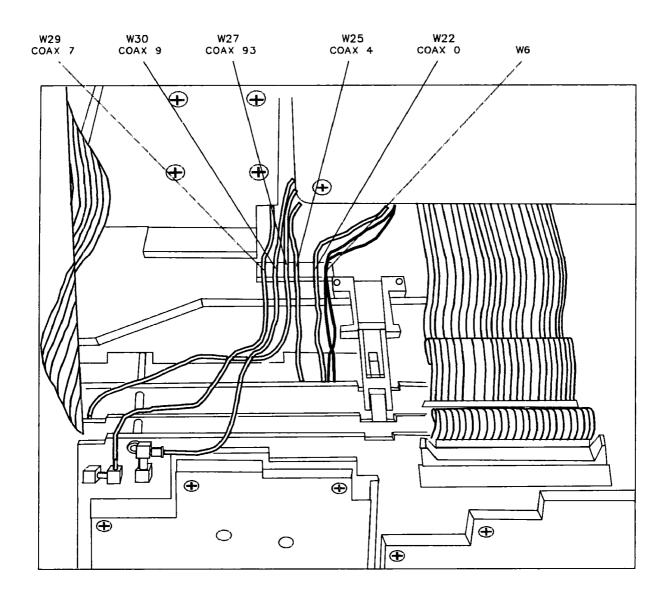
Figure 3-10. Coaxial Cable Clip
