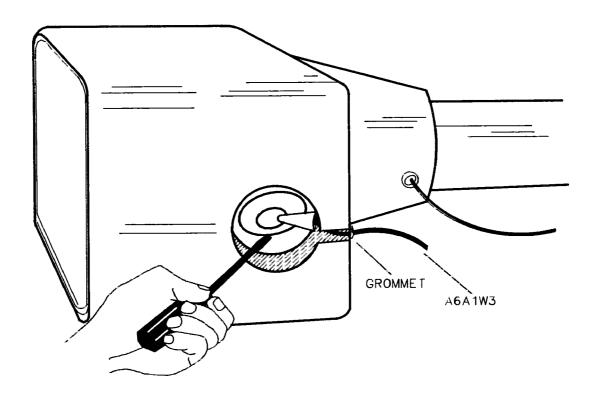
Figure 3-2. Grounding the Post-Accelerator Cable
