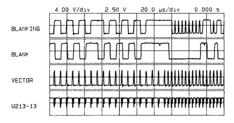
Figure 10-3. Blanking Waveforms
