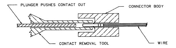
Figure 3-29. W3 Cable Connector
