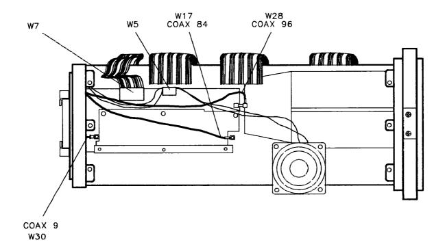
Figure 3-24. A16 Cable Routing
