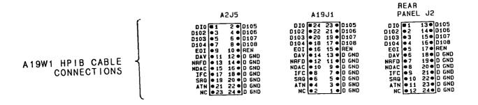
Figure 7-2 Ribbon Cable Connections (2 of 2)
