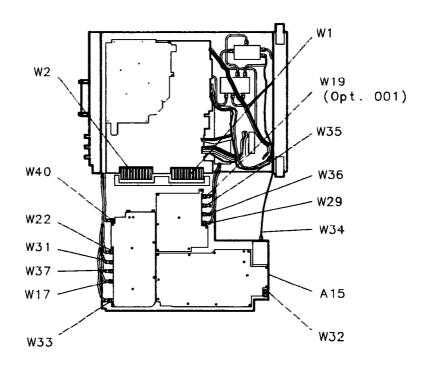
Figure 3-22. A14 and A15 Assembly Cables
