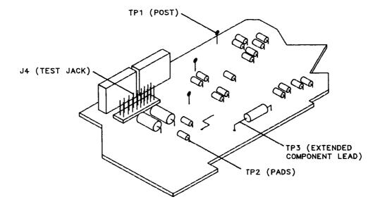
Figure 7-1. Assembly Test Points
