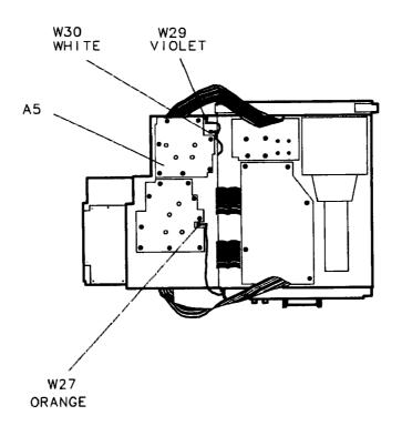
Figure 3-9. Assembly Cables (2 of 2)
