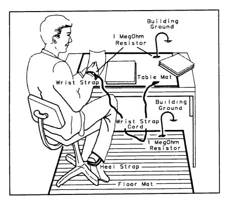
Figure 1-2. Example of a Static-Safe Work Station
