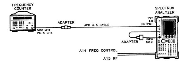
Figure 2-8. YTO Adjustment Setup
