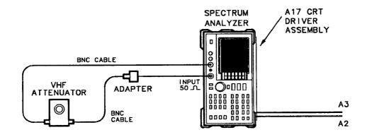
Figure 2-2. Display Adjustment Setup
