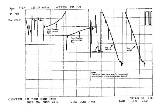
Figure 9-6. Detailed IF Adjust Signature (3)
