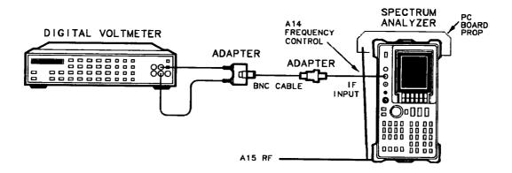
Figure 2-16. External Mixer Bias Adjustment Setup
