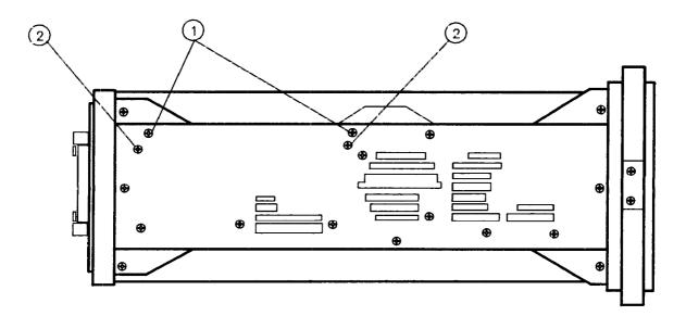
Figure 3-23. A16 and A17 Mounting Screws
