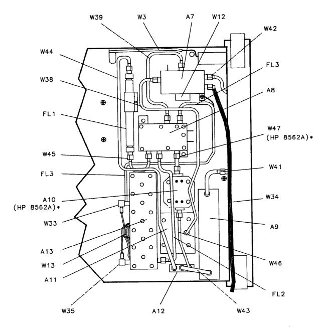
\* AT1 REPLACES A10 AND W47 IN HP8562B SPECTRUM ANALYZERS
