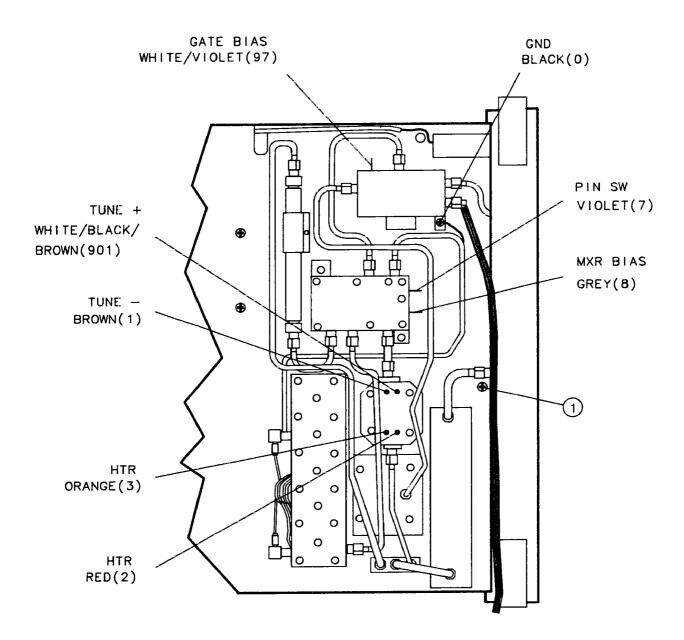
Figure 3-17. RF Section Bias Connections
