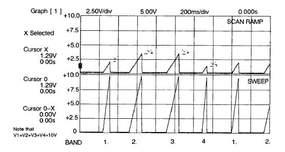
Figure 11-8. Sweep and Scan Ramps
