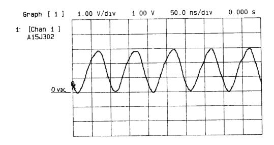
Figure 12-6. 10 MHz TTL Reference at U301 Pin 9
