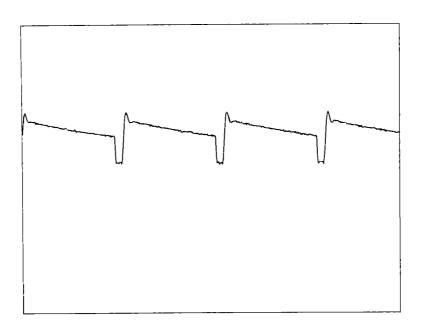
Figure 13-4. Buck Regulator Waveform
