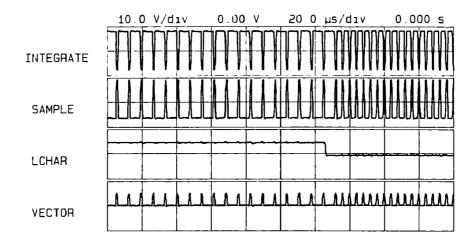
Figure 10-5. Switch Driver Waveform LCHAR
