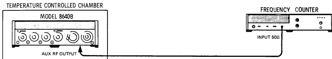
Figure 4-2. Frequency stability vs Temperature Test Setup
