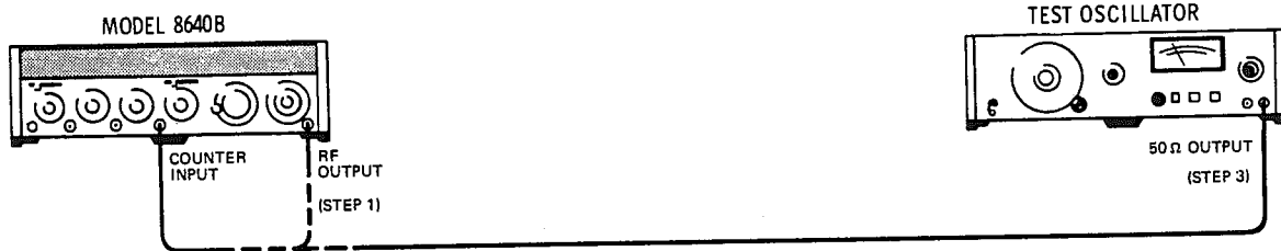
Figure 4-28. Counter External Sensitivity Test Setup
