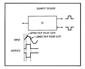
Figure 8-7. Schmitt Trigger
