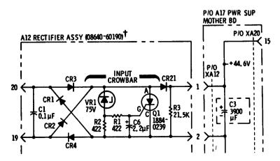
P/O Figure 8-74. Power Supply Circuits Schematic Diagram (P/O Change 1)
