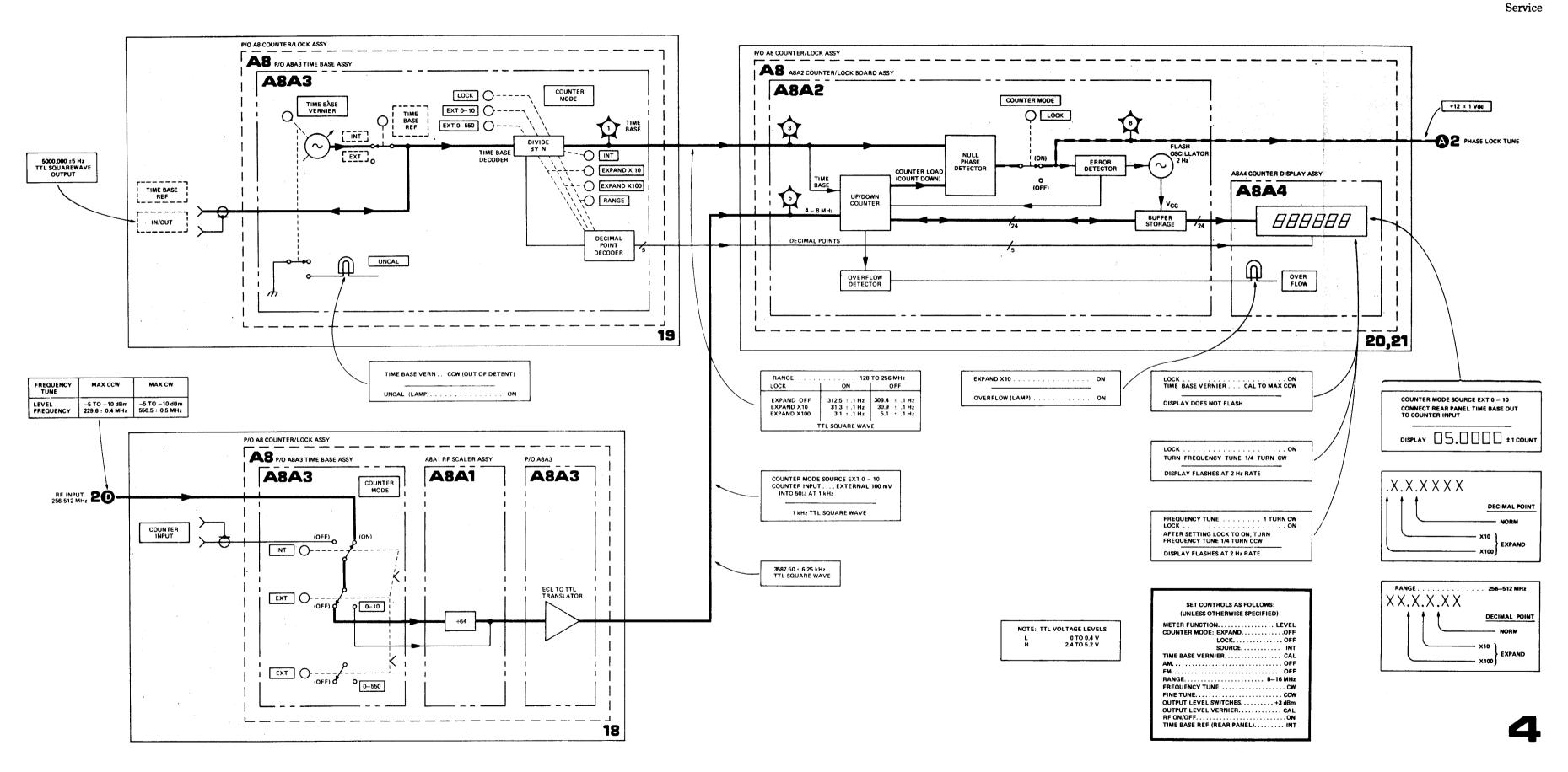
Figure 8-21. Counter/Lock Circuits Block Diagram
