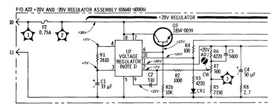
Figure 7-8. A22 +20V and -20V Regulator Assembly Backdating (Change I)
