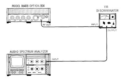
Figure 4-29. FM Distortion Test Setup
