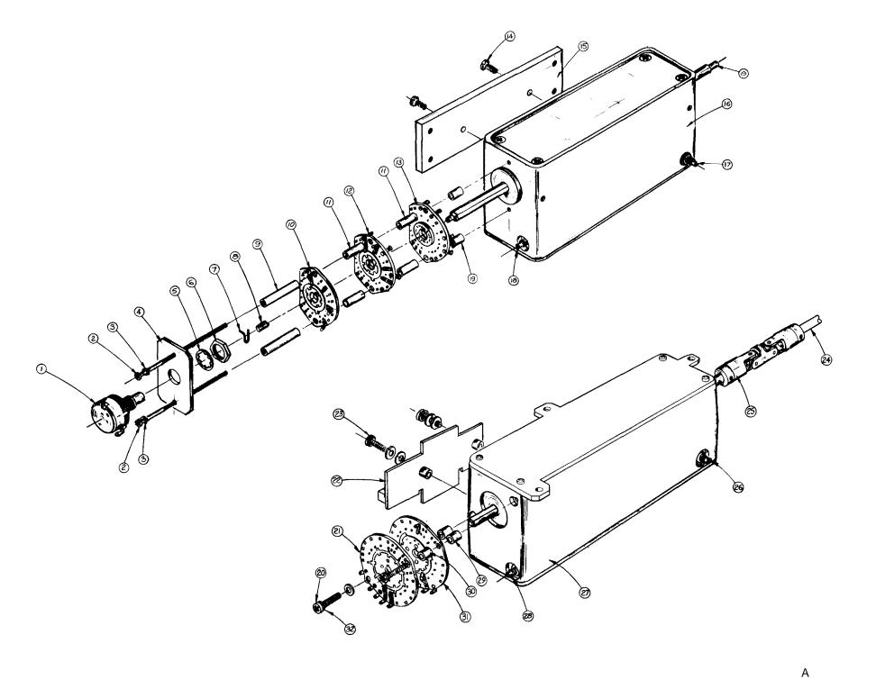
Figure 8-81. A1 and A19 Output Level Assemblies Illustrated Parts Breakdown
