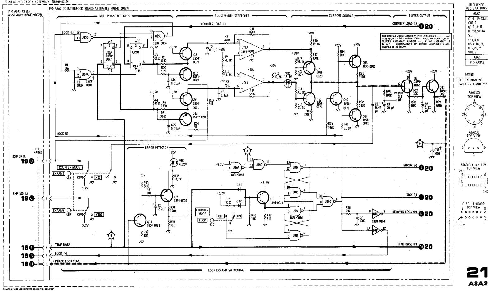
Figure 8-69. Counter Phase Lock Circuits Schematic Diagram
