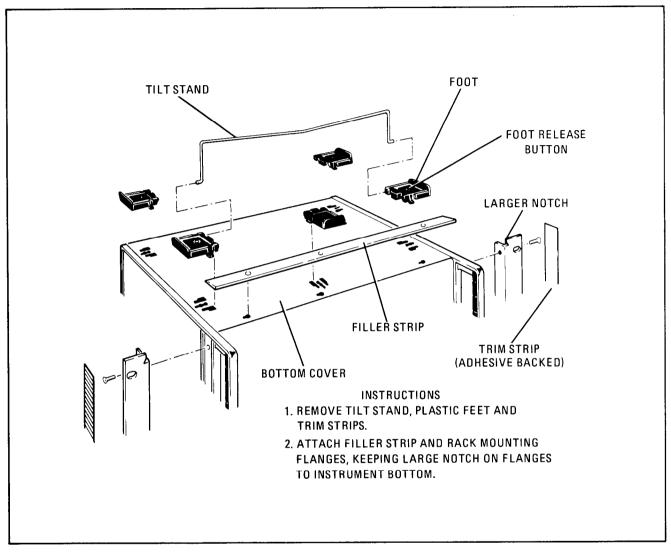
Figure 2-3. Preparation for Rack Mounting
