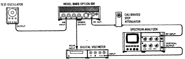
Figure 4-22. Demodulated Output Accuracy Test Setup
