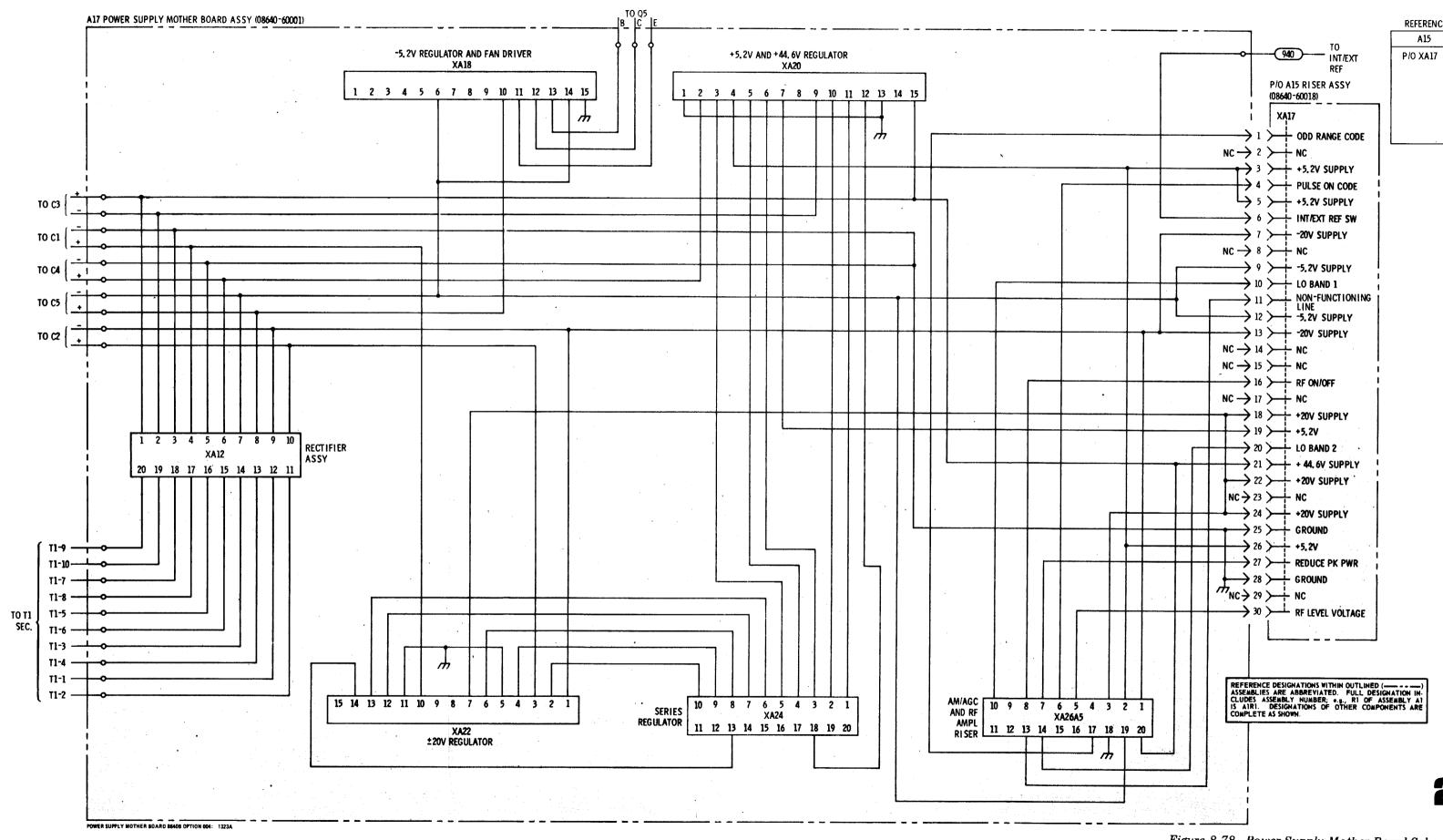
Figure 8-77. A17 Power Supply Mother Board Assembly Component Locations
