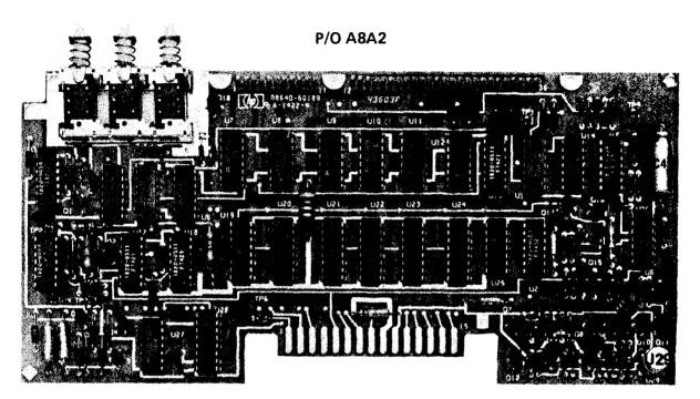
Figure 8-68. P/O A8A2 Counter/Lock Board Assembly Component Locations (P/O Change 1)
