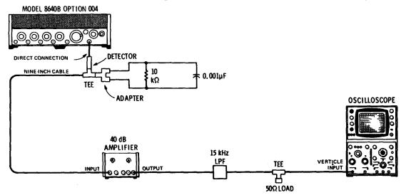
Figure 4-31. Incidental AM Test Setup
