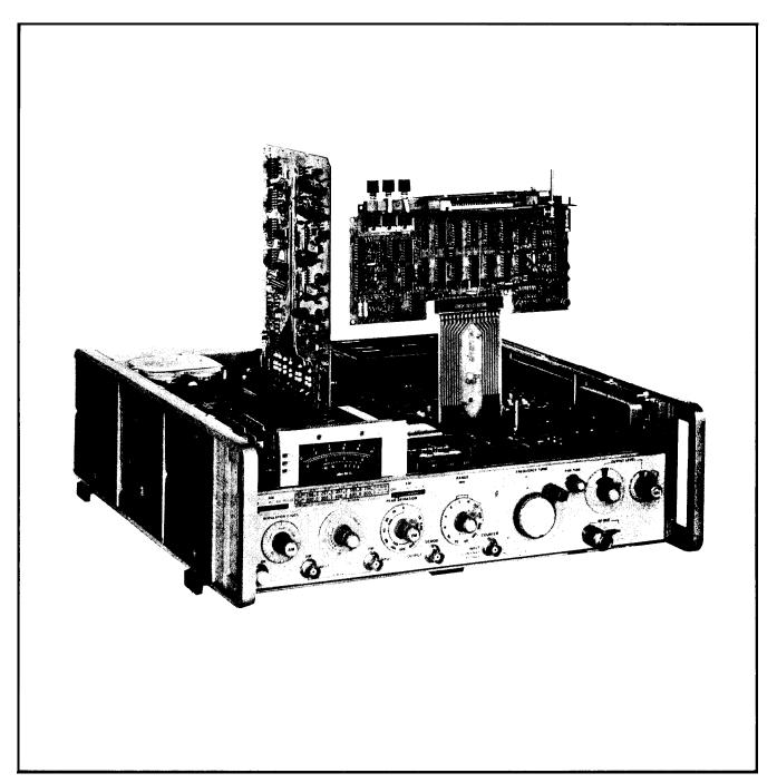
Figure 8-1. Signal Generator with Circuit Boards on Extenders
