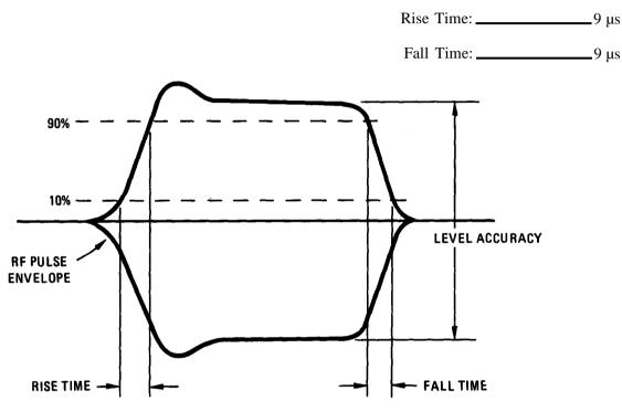
Figure 4-27. Pulse Measurements
