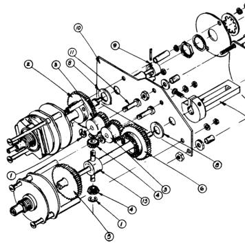
Figure 8-86. A9 Peak Deviation and Range Switch Assembly Illustrated Parts Breakdown
