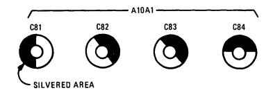
Figure 5-10. 256-512 MHz High Band Capacitor Adjustment Orientation
