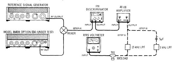
Figure 4-9. Residual FM Test Setup
