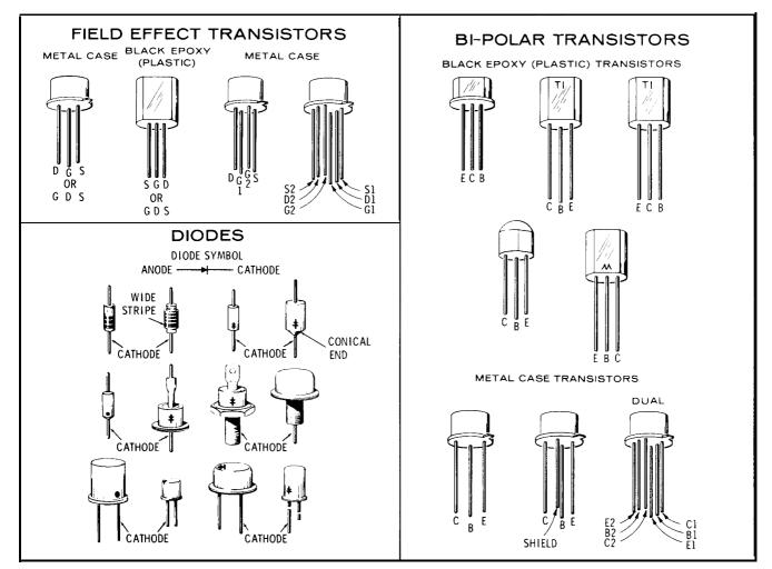
Figure 8-2. Examples of Diode and Transistor Marking Methods
