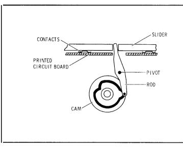
Figure 8-38. Action of RANGE Switch
