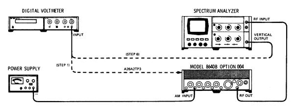
Figure 5-1. RF Detector Offset Adjustment Test Setup
