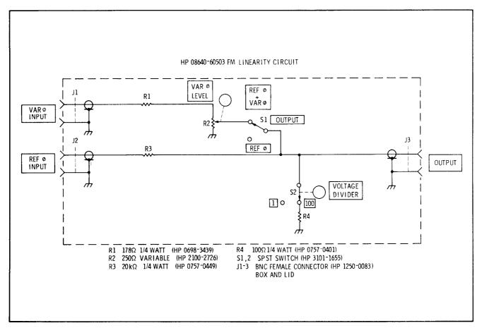
Figure 1-8. FM Linearity Circuit
