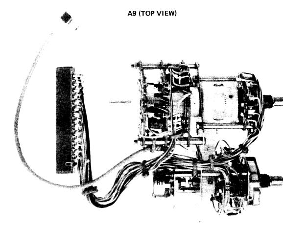
Figure 8-25. P/O A9 Peak Deviation and Range Switch Assembly Component Locations (1 of 2)
