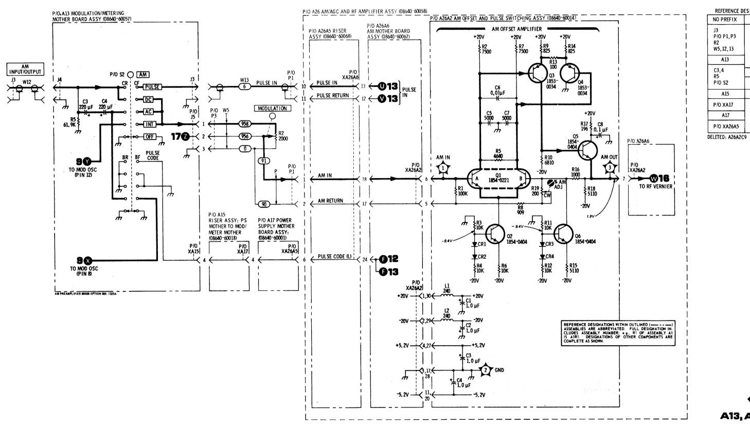
Figure 8-51. AM Preamplifier Schematic Diagram
