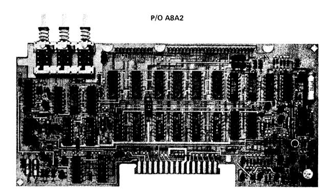
Figure 8-66. P/O A8A2 Counter/Lock Board Assembly Component Locations (P/O Change 6)
