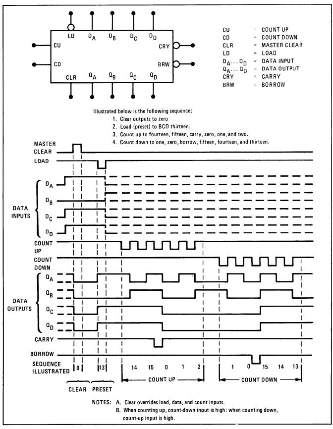
Figure 8-14. Programmable Up/Down Counter
