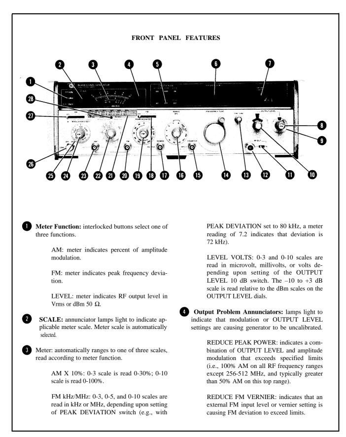
Figure 3-2. Front Panel Controls, Indicators, and Connectors (1 of 4)
