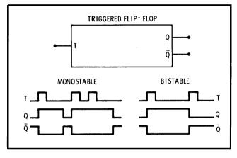
Figure 8-5. Triggered Flip-Flop
