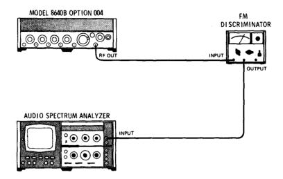
Figure 5-13. FM Linearity Adjustment (Alternate) Test Setup
