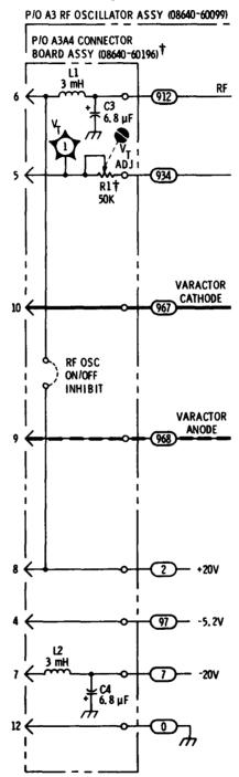
P/O Figure 8-23. RF Oscillator Simplified Diagram (P/O Change 2)
