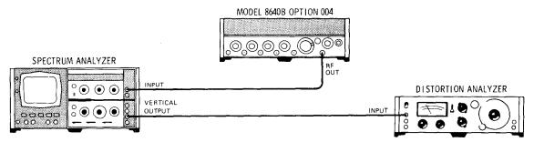
Figure 4-19. AM Distortion Test Setup
