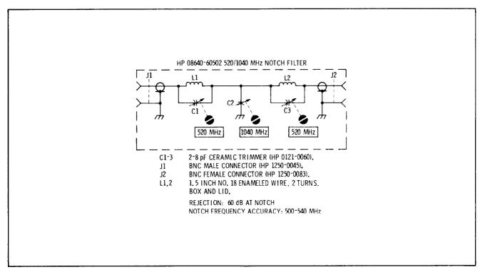
Figure 1-7. 520/1040 MHz Notch Filter
