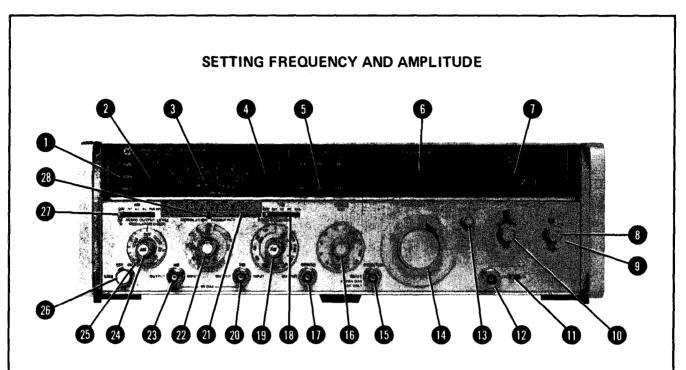
is read on the indicated voltage scale. At approximately 1 on the 0-3 scale, or 3 on the 0-10 scale, the meter autoranges to the next lower range. The vernier provides additional attenuation and also affects meter autoranging.
