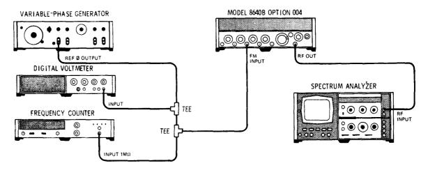
Figure 5-14. FM Sensitivity Adjustment Test Setup
