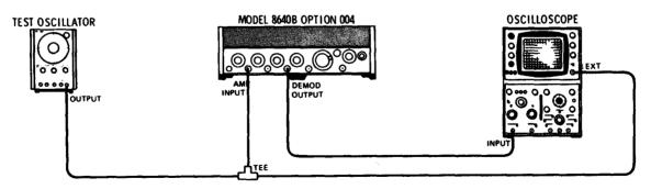
Figure 4-23. AM Phase Shift Test Setup
