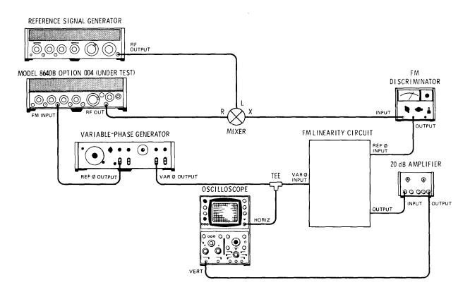
Figure 5-11. FM Linearity Adjustment Test Setup
