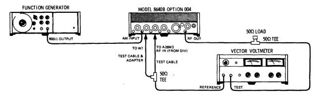
Figure 4-21. Peak Incidental Phase Modulation Test Setup
