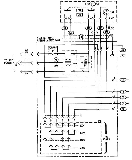
Figure 7-7. Power Supply Circuits Backdating (Change I)
