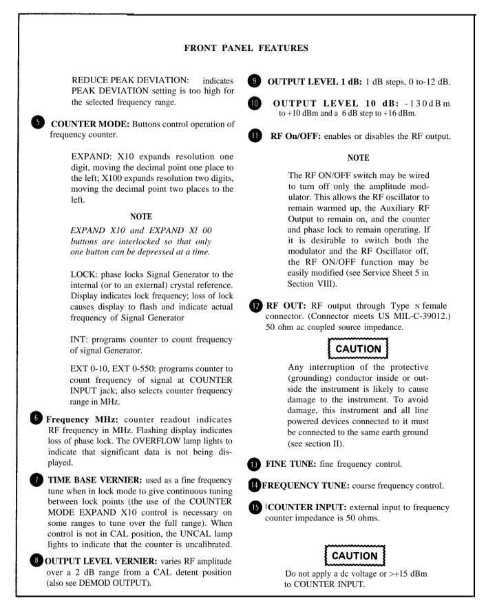
Figure 3-2. Front Panel Controls, Indicators, and Connectors (2 of 4)
