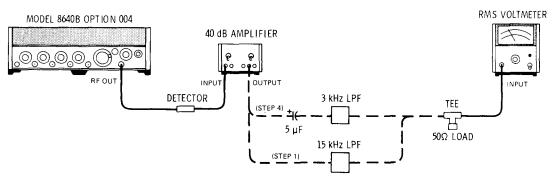
Figure 4-8. Residual AM Test Setup
