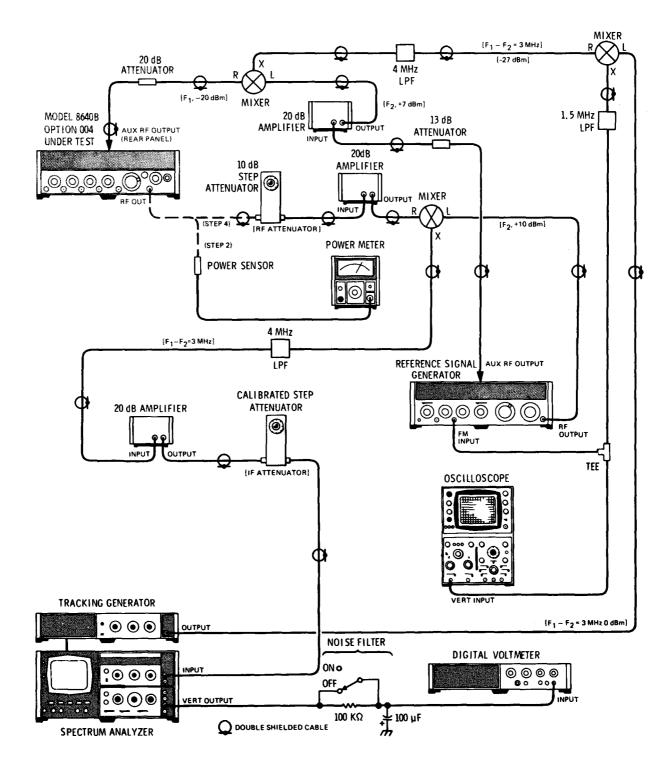
Figure 4-11. Output Level Accuracy Test Setup (Complete)
