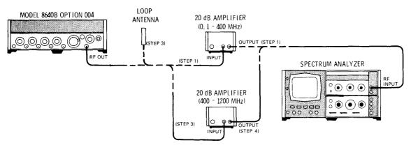
Figure 4-15. Output Leakage Test Setup
