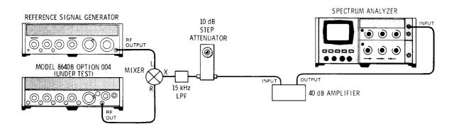
Figure 4-7. Single Sideband Broadband Noise Floor Test Setup
