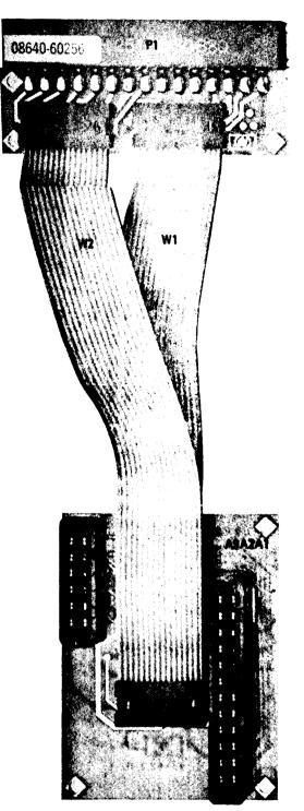
Figure 8-25B. A9A2 Interconnect Assembly Component Locations (P/O Change 7)
