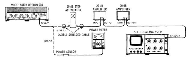
Figure 4-10. Output Level Accuracy Test Setup (Abbreviated)
