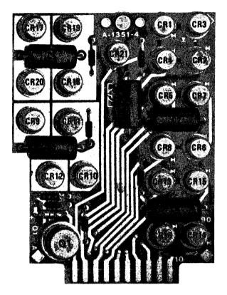
Figure 8-71. A12 Rectifier Assembly Component Locations (P/O Change 1)
