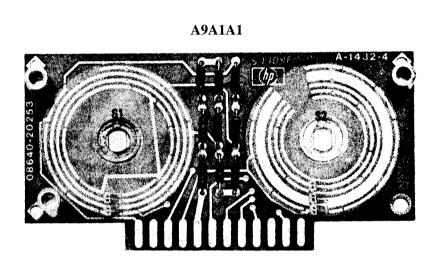
Figure 8-31A. A9A1A1 Peak Deviation Band Switch Board Assembly Component Locations (P/O Change 7)
