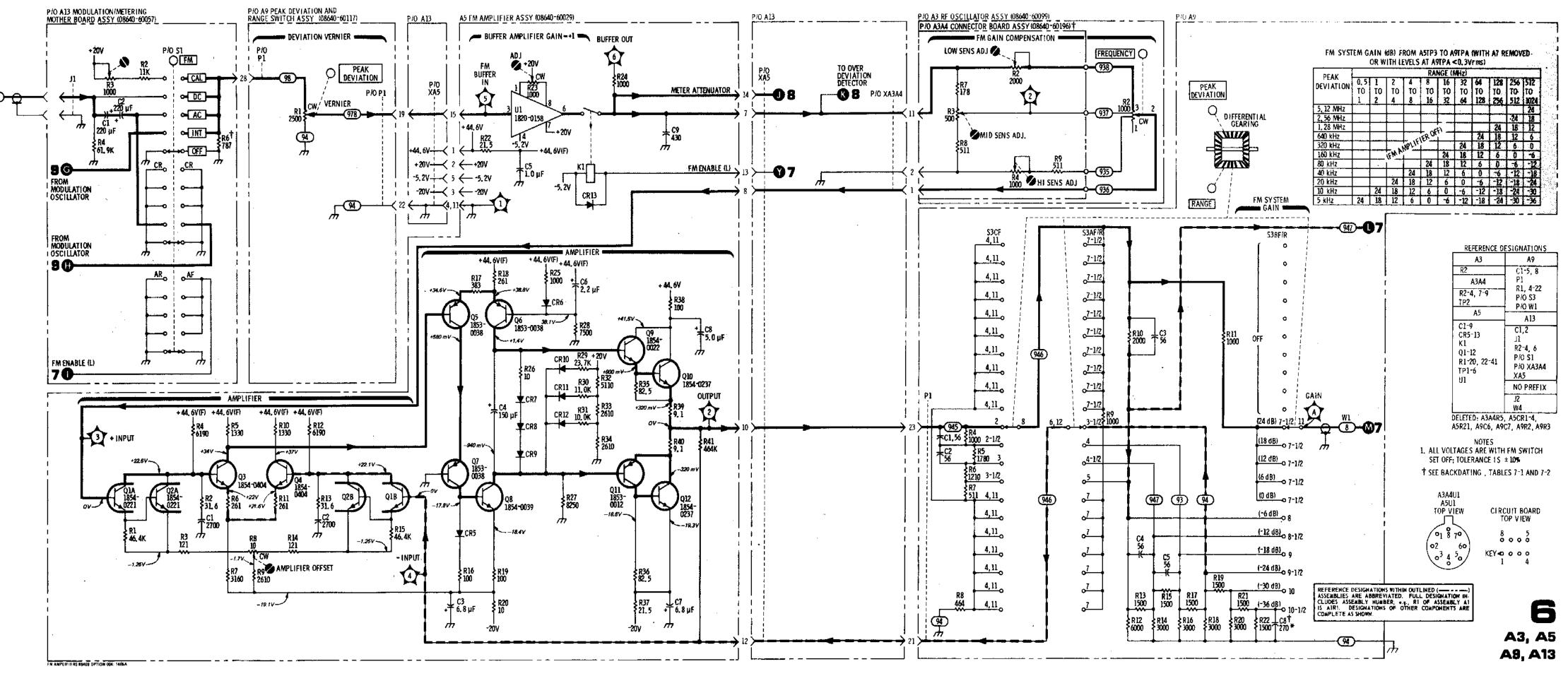
Figure 8-27. FM Amplifiers Schematic Diagram
