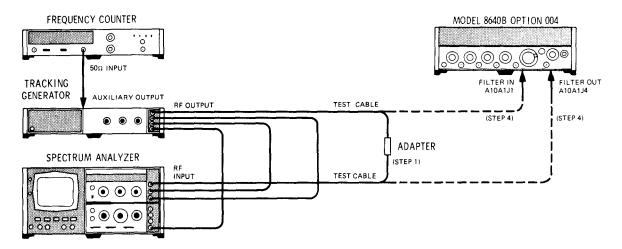
Figure 5-9. RF Filter Adjustment Test Setup
