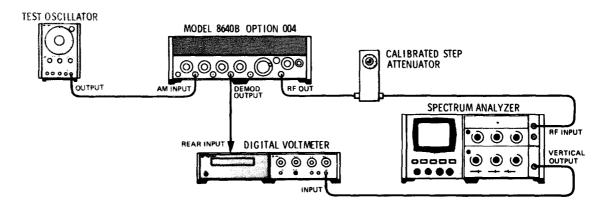
Figure 5-4. AM Accuracy Adjustment Test Setup
