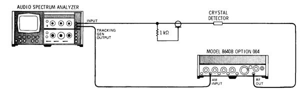
Figure 4-18. AM 3 dB Bandwidth Test Setup
