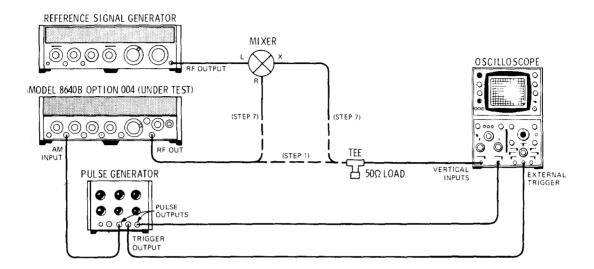
Figure 4-26, Pulse Modulation Test Setup
