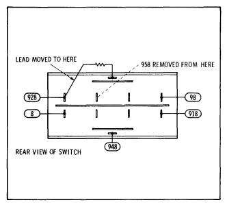
Figure 7-9. Modified Line Switch Wiring
