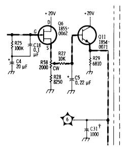
P/O Figure 8-69. Counter Phase Lock Schematic Diagram (P/O Change 6)
