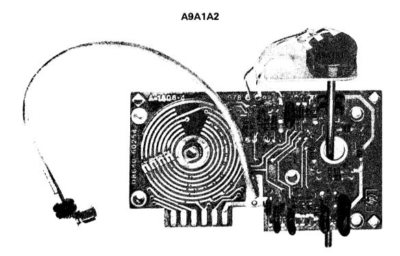
Figure 8-25A. A9A1A2 FM Gain Switch Board Assembly Component Locations (P/O Change 7) A9A2
