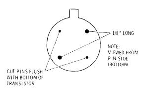
Figure 8-82. RF Oscillator Transistor Preparation
