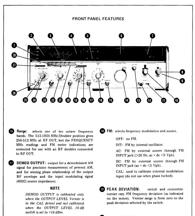
An internal switch controls the level of the DEMOD OUTPUT signal. Refer to Figure 3-3. **FM INPUT/OUTPUT:** 600 ohm input for external FM; nominally 1 Vpk (0.7071 Vrms) required for full peak deviation selected by PEAK
