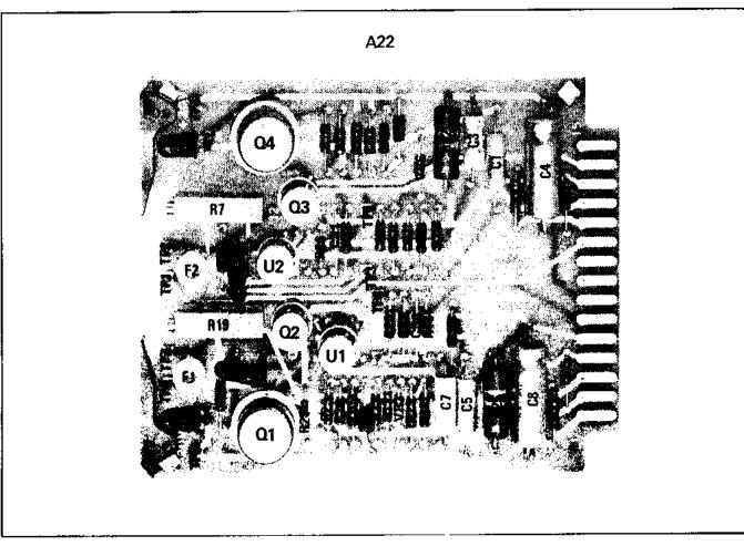
Figure 8-73. A 22 +20V and 20V Regulator Assembly Component Locations
