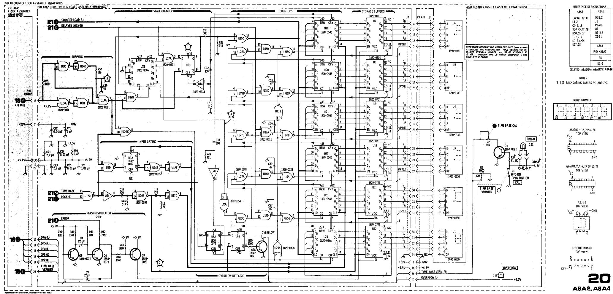
Figure 8-67. Up/Down Counter and Display Schematic Diagram
