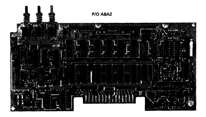
Figure 8-66. P/0 A8A2 Counter/Lock Board Assembly Component Locations (P/O Change 1)
