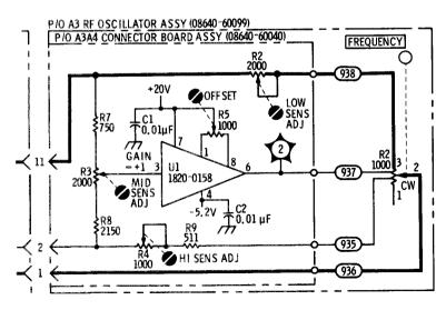
Figure 7-4. A3A4 Connector Board Assembly Backdating (Change G)
