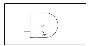
Figure 8-3. Open Collector Output Stage (AND Gate)
