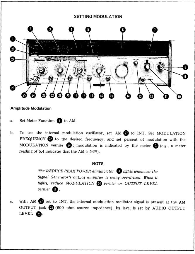
Figure 3-7. Setting the Modulation Controls (1 of 5)
