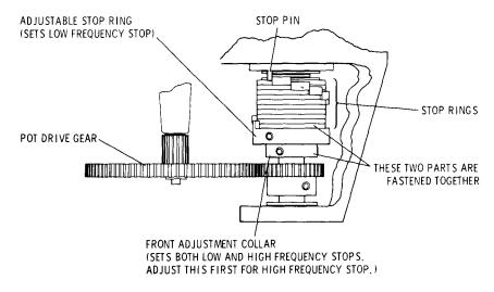
Figure 5-6. Location of RF Oscillator Stop Adjustments. Shown in Maximum ccw Position. Top View with Instrument Upside Down.
