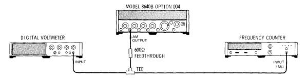
Figure 4-16. Internal Modulation Oscillator Test Setup
