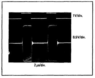
Figure 1-5. Pulsed RF 20 MHz Carrier Frequency at 400 kHz Pulse Rate and 1 µs Pulse Width.
