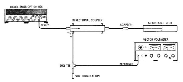
Figure 4-13. Output Impedance Test Setup (Signal Frequency)
