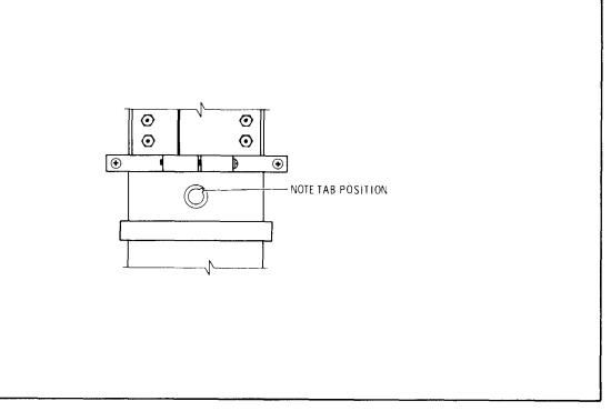
Figure 8-83. RF Oscillator Transistor Orientation
