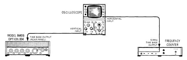
Figure 5-15. Internal Reference Frequency Adjustment Test Setup
