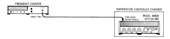
Figure 4-33. Internal Reference Accuracy Test Setup
