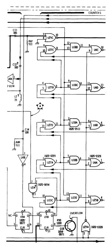
P/O Figure 8-67. Up/Down Counter and Display Schematic Diagram (P/O Change 6)
