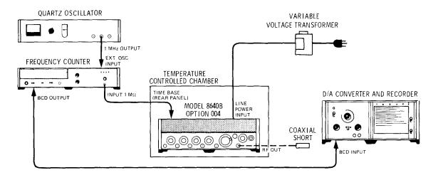
Figure 4-34. Internal Reference Drift Rate (Stability) Test Setup
