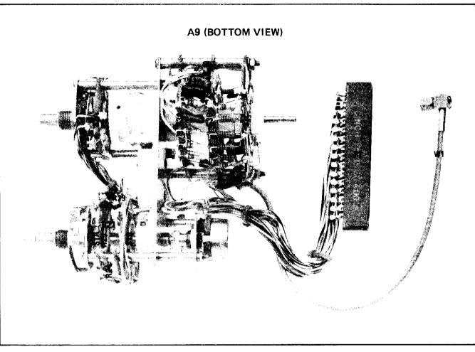
Figure 8-31. P/O A9 Peak Deviation and Range Switch Assembly Component Locations (2 of 2)
