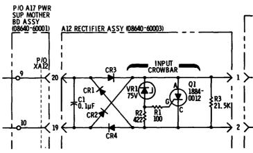
Figure 7-3. A12 Rectifier Assembly Backdating (Change C)
