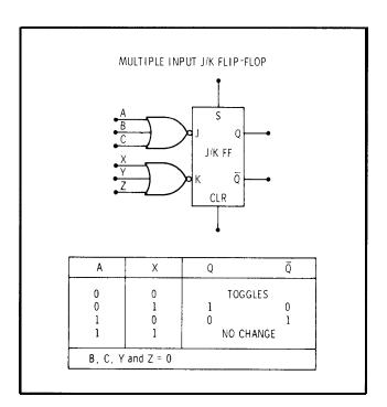
Figure 8-9. Multiple Input J/K Flip-Flop
