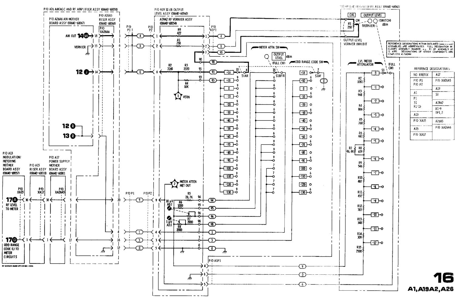
Figure 8-55. RF Vernier Schematic Diagram
