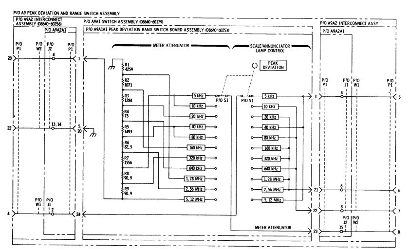
P/O Figure 8-33. Over-Deviation Detector and Meter Control Circuits Schematic Diagram (P/O Change 7)
