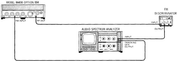
Figure 4-28. FM 3 dB Bandwidth Test Setup
