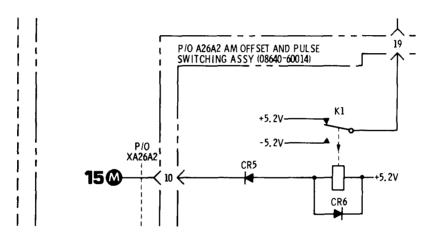
Figure 7-1. A26A 2 AM Offset and Pulse Switching Assembly Backdating (Change C)
