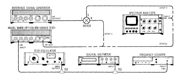
Figure 4-30. FM Sensitivity and Accuracy Test Setup
