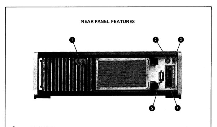
AUX RF OUTPUT: nominal -5 dBm auxiliary RF output; 500 ohm source impedance. Signal does not contain amplitude or pulse modulation (however, it does contain FM). On the 512-1024 MHz/Doubler Band the auxiliary RF output is one-half the frequency of the indicated RF frequency.
