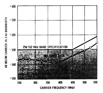
Figure 1-3. Specified Signal-to-Phase Noise Ratio at 20 kHz Offset vsus Carrier Frequency (MHz). (Stated in a 1 Hz Bandwidth.) For lower bands, phase-noise decreases approximately 6 dB per frequency division down to the broadband noise floor.
