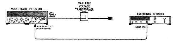
Figure 4-3. Frequency Stability vs Line Voltage Test Setup
