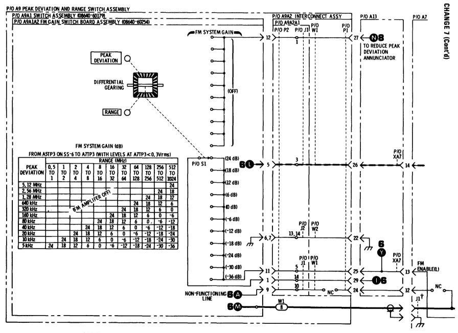
P/O Figure 8-29. FM Shaping Circuits and Phase Lock Loop Filter Schematic Diagram (P/O Change 7)
