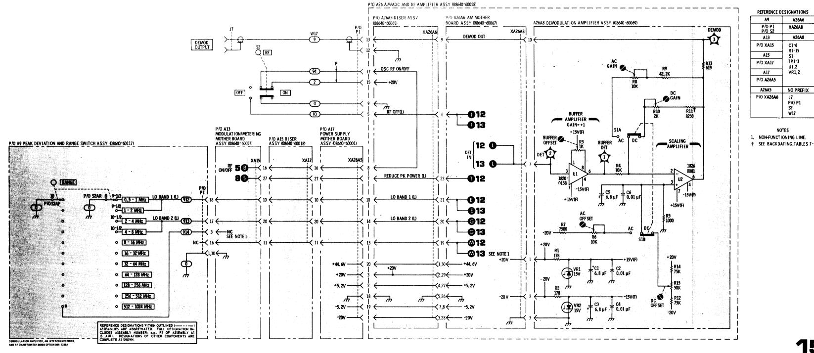
Figure 8-53. AM Interconnections, RF ON/OFF Switch and Demodulation Amplifier Schematic Diagram
