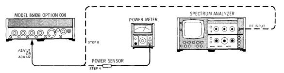
Figure 5-7. RF Oscillator Output Power Adjustment Test Setup
