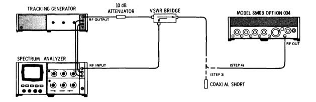
Figure 4-14. Output Impedance Test (Broadband)
