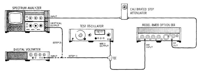
Figure 4-20. AM Sensitivity and Accuracy Test Setup
