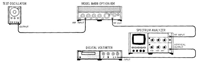
Figure 4-25. AM Flatness Test Setup
