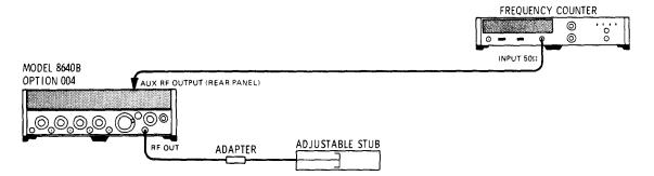
Figure 4-4. Frequency Stability us Load, Level, and Mode Test Setup
