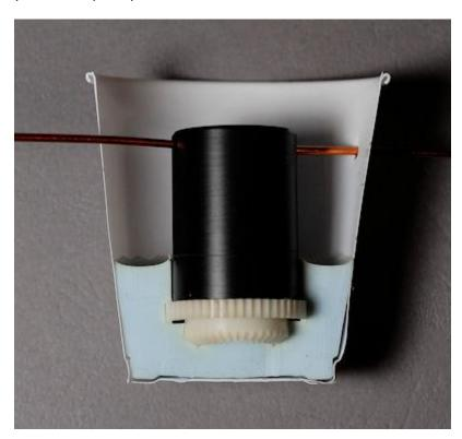
Using the scale, mix about 1 oz of RTV1000 in another plastic cup. Mix thoroughly and put the cup in the vacuum chamber. Pump it down to degas the mixture. It will foam up, and can easily overflow the cup, so bring the pressure down at a rate that keeps the material in the cup. A note about my vacuum
