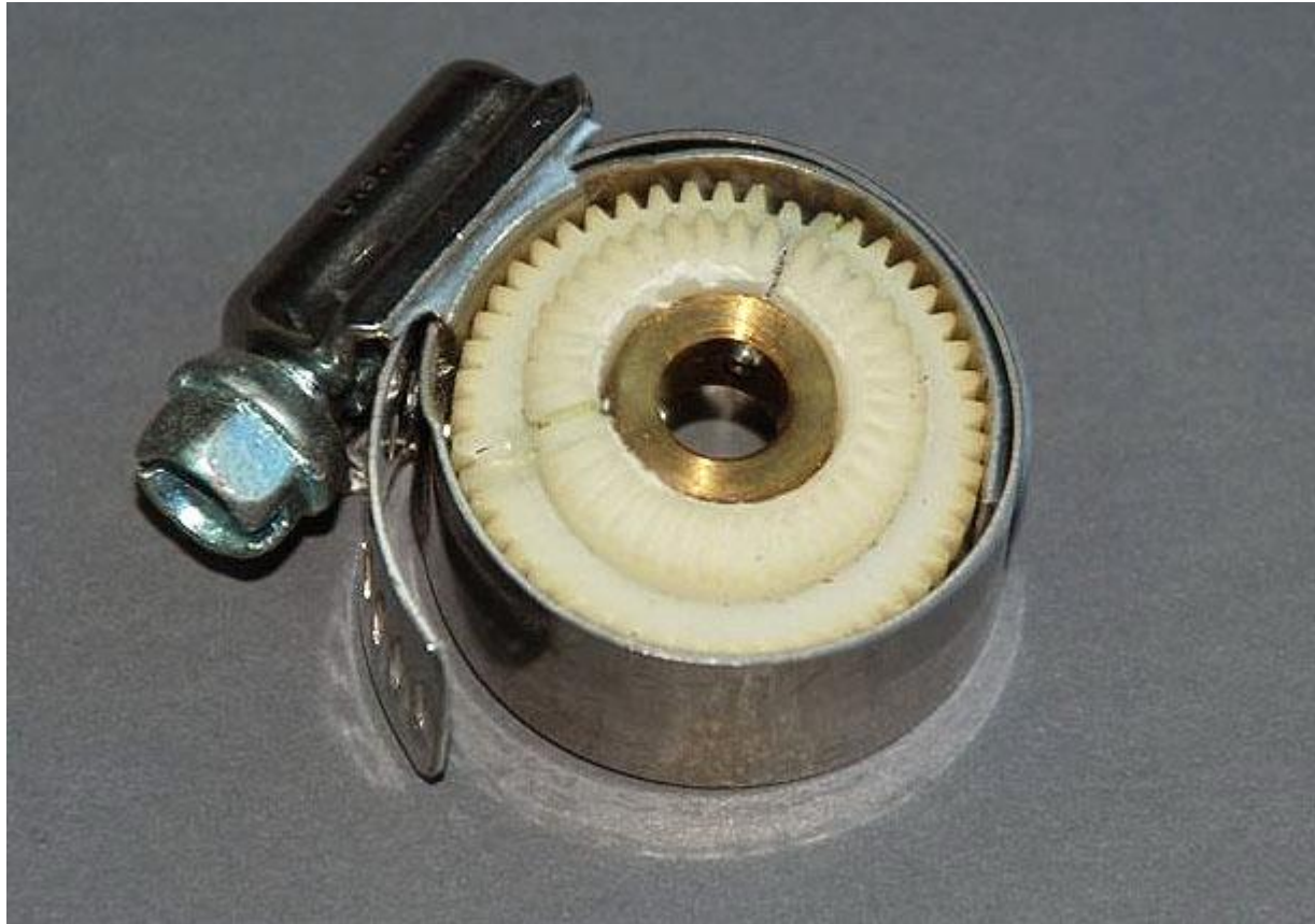
Fig 7. Hose clamp holding gear together while glue sets
