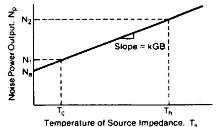
Figure 3. Available noise power and noise figure measurement.
