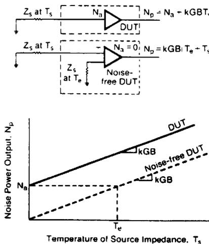
Figure 2. Available noise power & effective input noise temperature.
